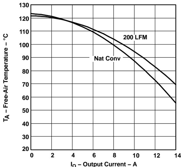
Figure 17. TPS54010 Safe-Operating Area with Airflow
