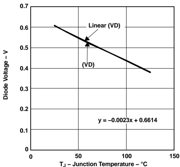
**Figure 8. TPS54610 Diode Voltage vs Junction Temperature**
