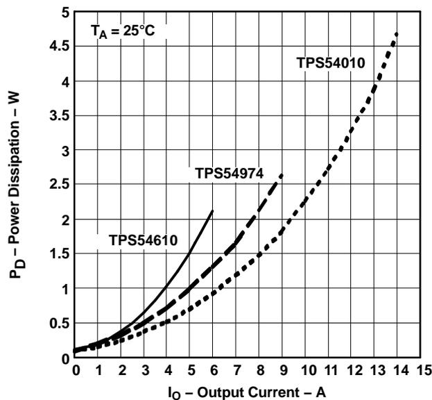
**Figure 11. Device Power Dissipation vs Output Current**
