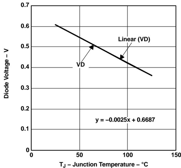
Figure 10. TPS54010 Diode Voltage vs Junction Temperature
