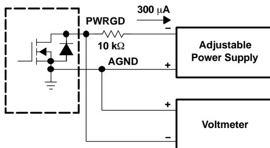
Figure 7. Test Setup
