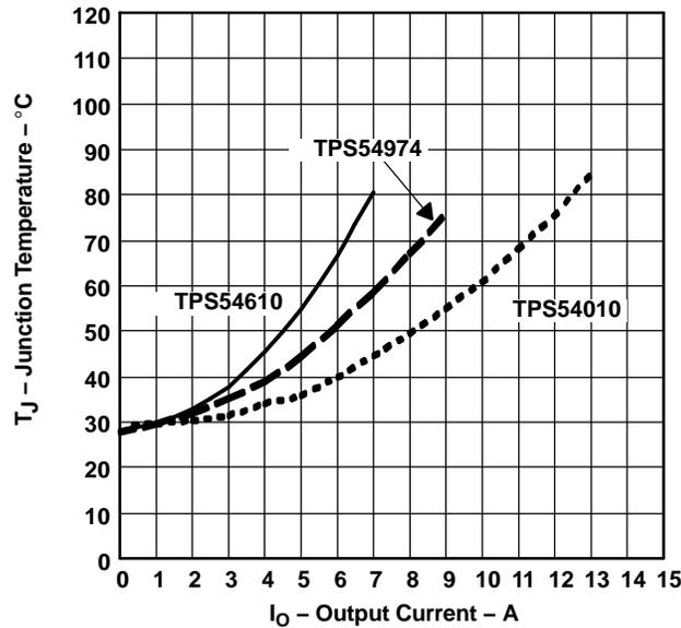
**Figure 12. Device Junction Temperature vs Output Current**
