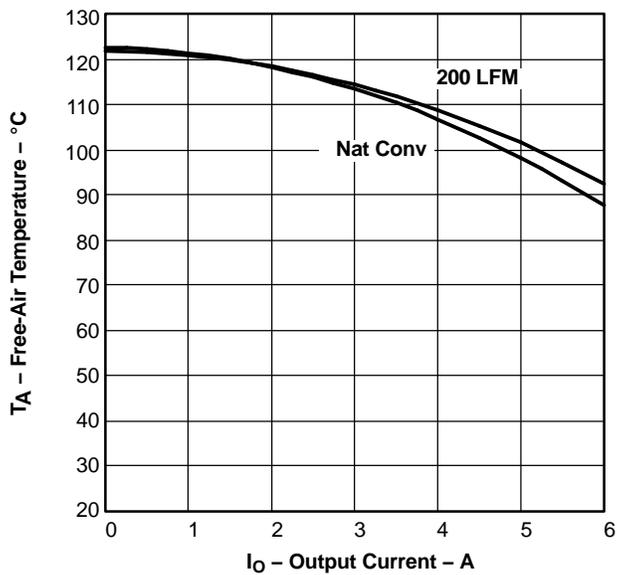
Figure 15. TPS54610 Safe-Operating Area with Airflow
