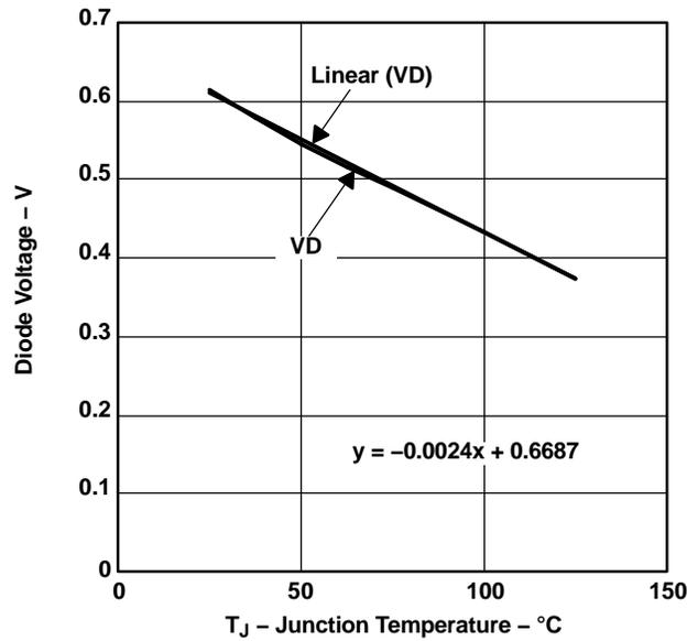
Figure 9. TPS54974 Diode Voltage vs Junction Temperature
