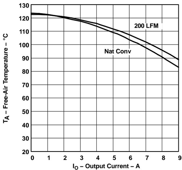
Figure 16. TPS54974 Safe-Operating Area with Airflow
