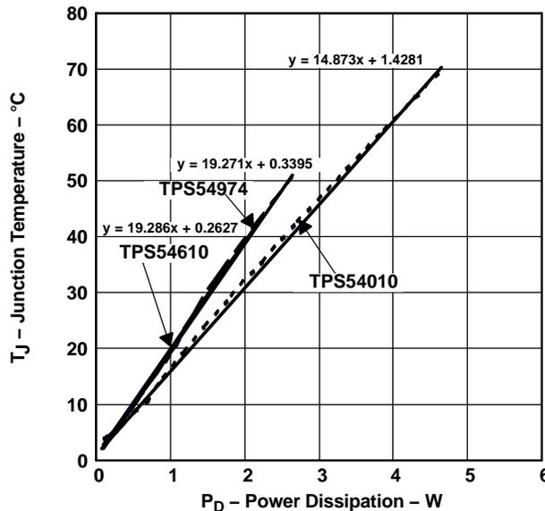
**Figure 13. Junction Temperature Rise vs Device Power Dissipation**
