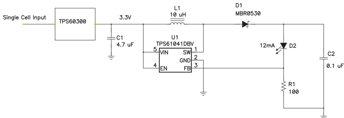
**Figure 1. Single Cell Operation With Intermediate Voltage Conversion**
