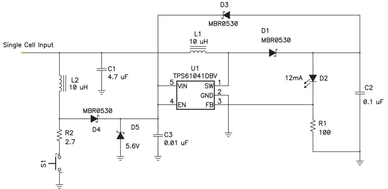
**Figure 3. Single Cell Operation With Push-Button Startup**
