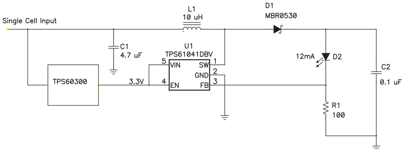
**Figure 2. Single Cell Operation With Auxiliary Bias Voltage**
