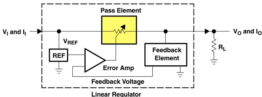
Figure 1. Potentiometer Model of a Linear Regulator
