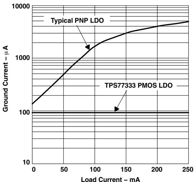
**Figure 7. Comparison of 100- $\mu$ A  $I_Q$  PMOS and PNP LDOs**
