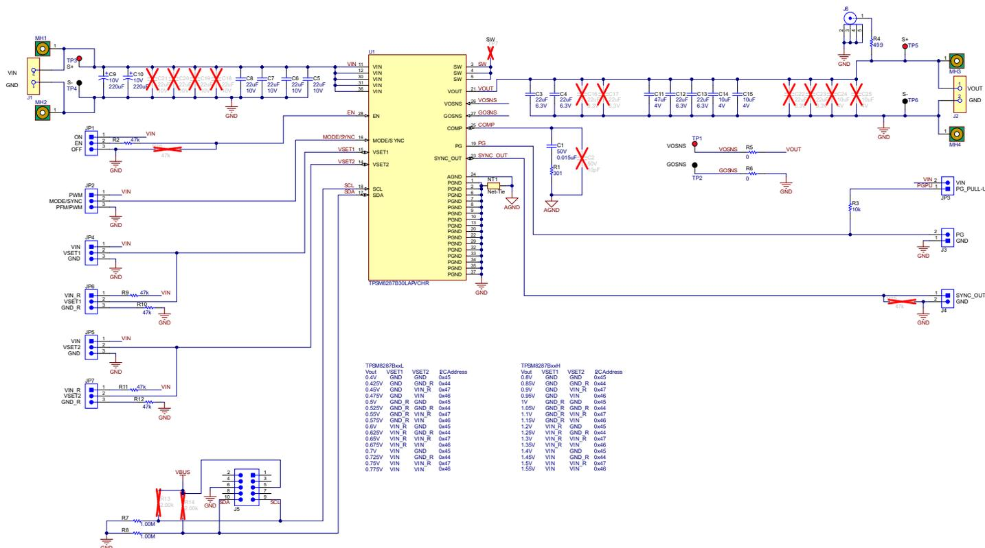
Figure 5-1. TPSM8287B30LAPEVM Schematic
