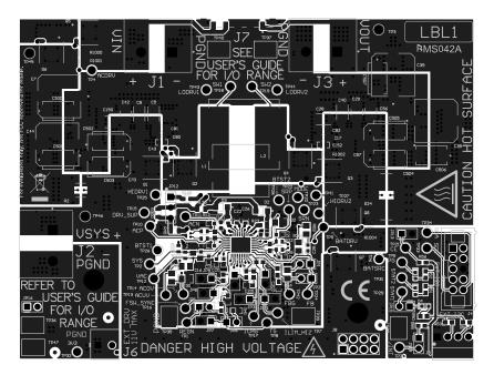
Figure 3-2. Top Layer and Overlay
