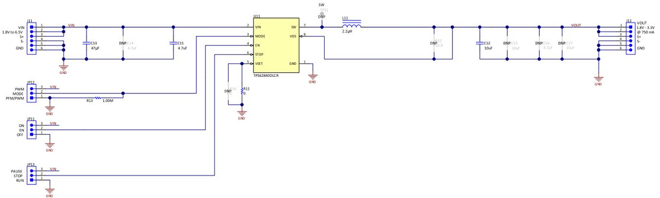
Figure 11. TPS62840 Schematic
