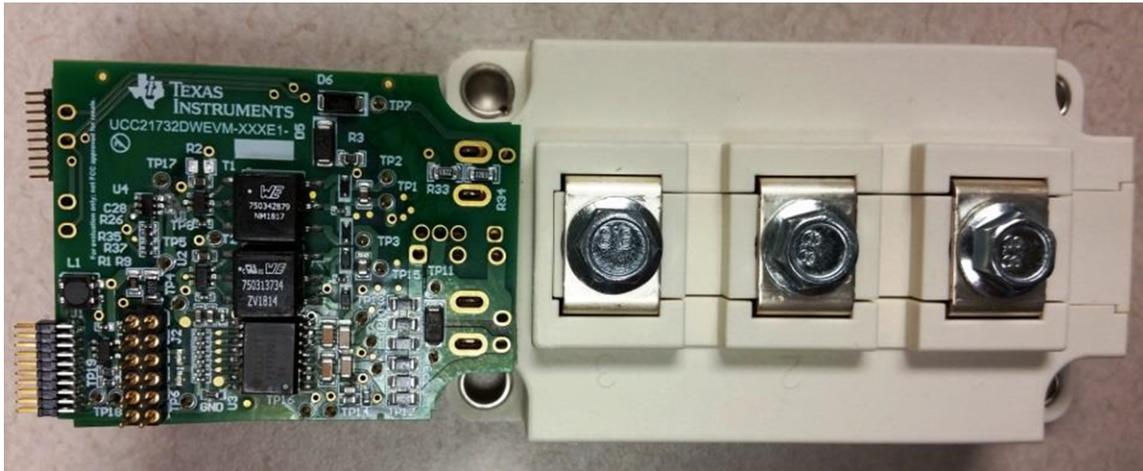
In 106-mm half-bridge module configuration two boards are placed one on top of another and the bottom board is flipped over. The supply voltage and input signals are provided through connectors J1 on each board. By connecting IN+ and INE- terminals on one board to INE+ and IN- terminals accordingly on another board, the overlapping protection circuit using logic U5 is engaged. This circuit could be disabled by removing resistors R31 and R32 in case of overlapping is required in the system.
