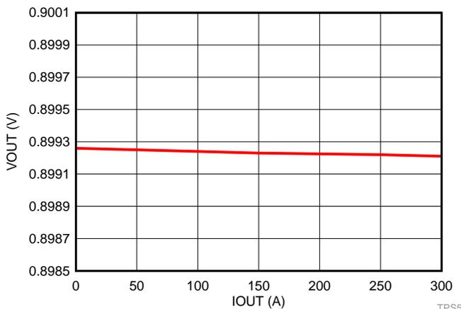
V<sub>OUT</sub> = 0.9 V, V<sub>IN</sub> = 12 V
