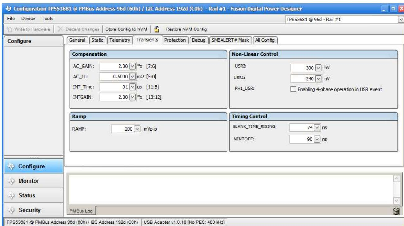
Figure 48. Transients Configure Tab
