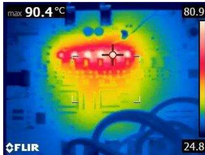
A V<sub>IN</sub> = 12 V, V<sub>OUT</sub> = 0.9 V, I<sub>OUT</sub> = 294A
