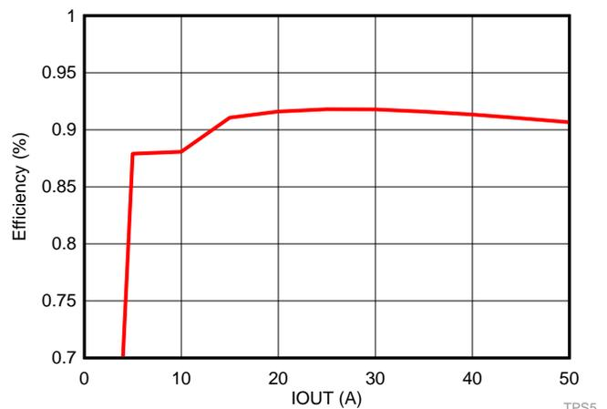
V<sub>OUT</sub> = 0.8 V, V<sub>IN</sub> = 12 V
