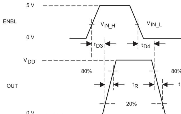
indent: The 20% and 80% thresholds depict the dynamics of the bipolar output devices that dominate the power MOSFET transition through the Miller regions of operation.
