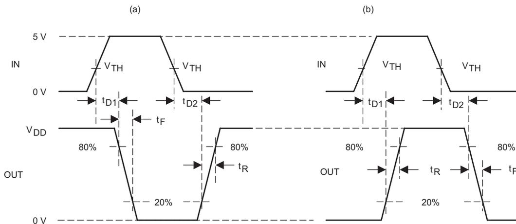
indent: The 20% and 80% thresholds depict the dynamics of the bipolar output devices that dominate the power MOSFET transition through the Miller regions of operation.
