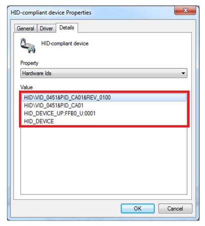
Figure 8. USB Interface Hardware IDs
