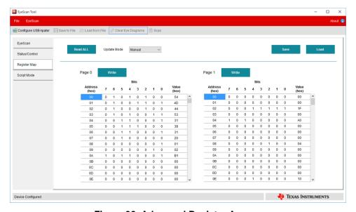
Figure 32. Advanced Register Access
