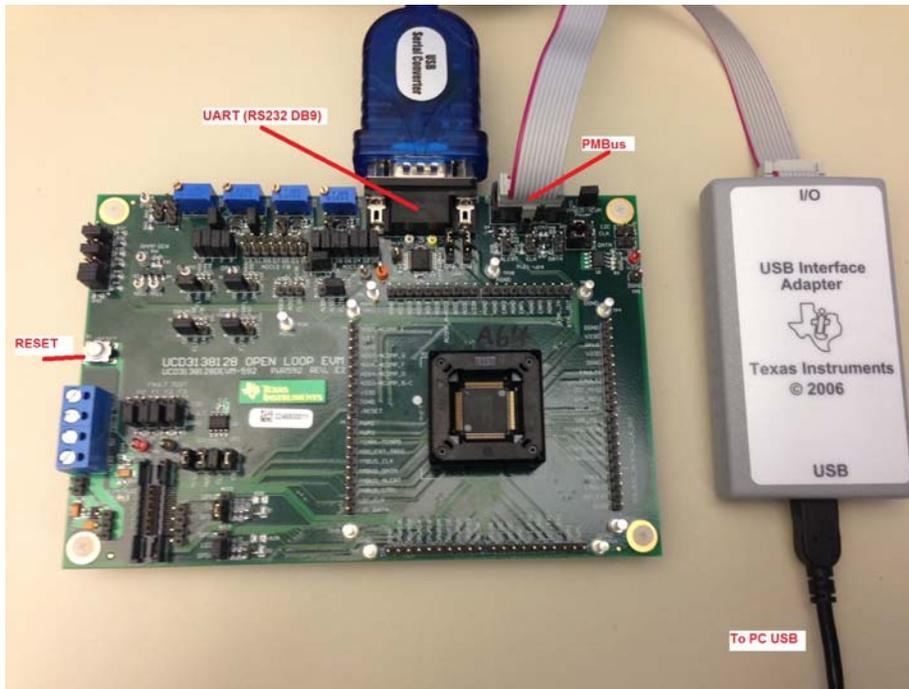
Figure 12. UCD3138A64OEV-662 Test Connections
