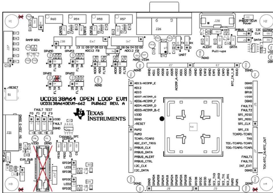
Figure 15. UCD3138A64OEVM-662 Top Layer Assembly Drawing (Top view)
