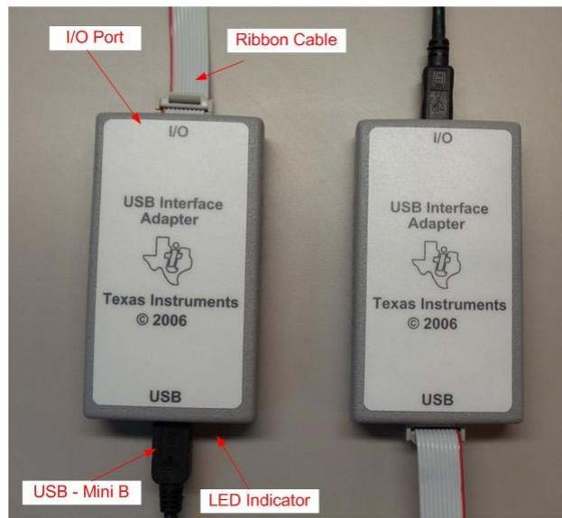
Figure 11. USB-to-GPIO Interface Adapter (HPA172) Outlook.
