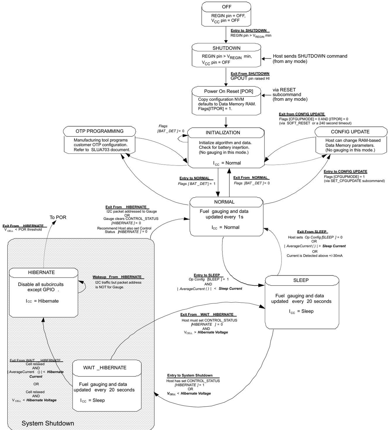
Figure 2-1. Operating Modes Diagram
