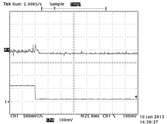
Figure 11. 0.1-A to 0.6-A Load Step
