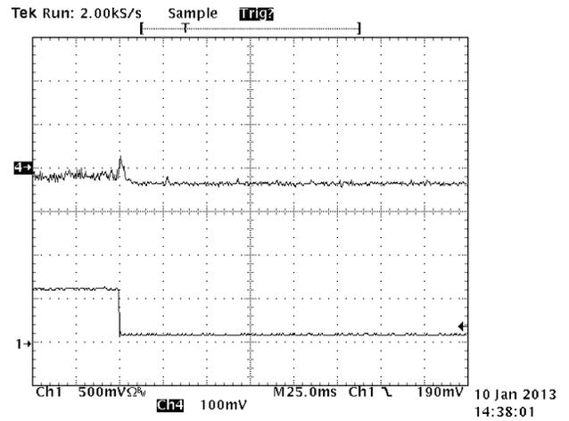
Figure 9. 0.1-A to 0.6-A Load Step
