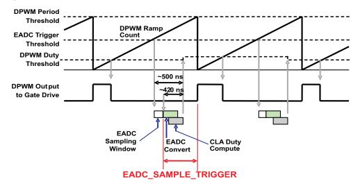
Figure 1. EADC Sample Trigger Timing
