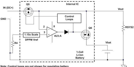
Note: Control loops are not shown for regulating battery constant current/voltage or Battery Supplement mode.
