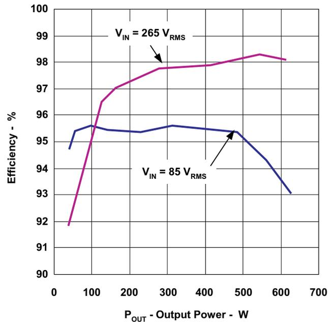
Figure 3. Efficiency at 85 VRMS and 265 VRMS
