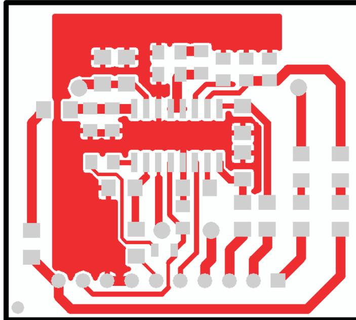
Figure 16. PR735 Controller Board Layout (viewed from top)
