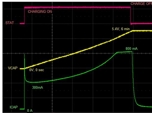
**Figure 1. Charging Two 50-F Supercapacitors in Series to 5.4 V with the BQ25173**
