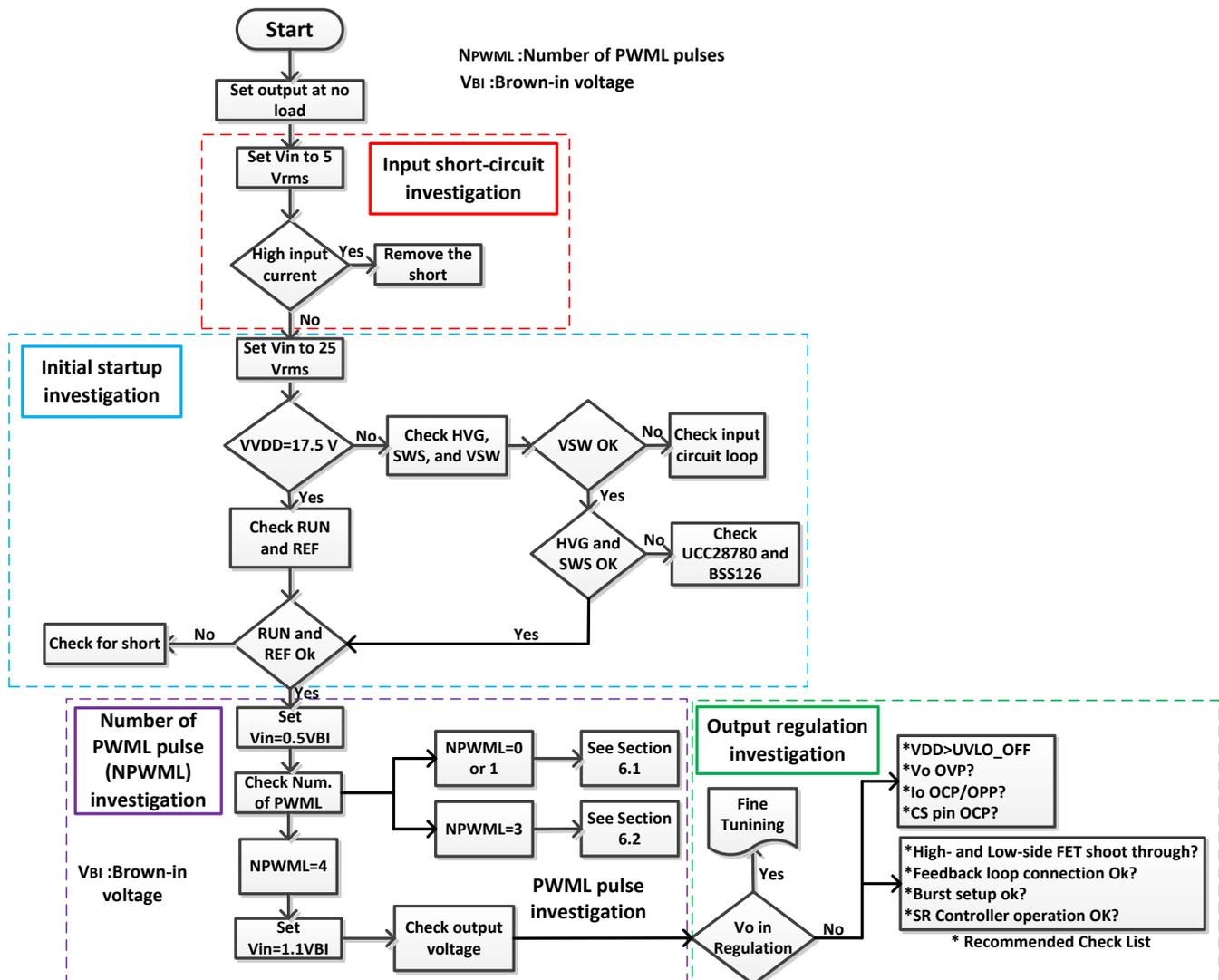
Figure 2. A Procedural Debugging Flowchart for Power-up Process
