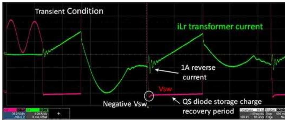
Figure 16.  $V_{SW}$  and Transformer Primary Current During Transient
