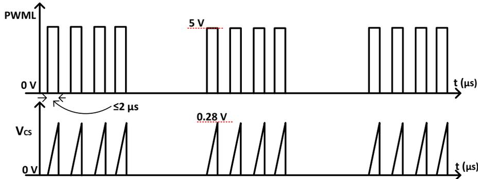
Figure 6. PWML Waveform Along with  $V_{CS}$  When Four PWML Pulses Are Observed
