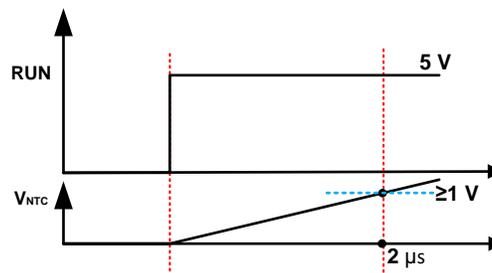
Figure 10. RUN and Voltage Across the NTC Pin
