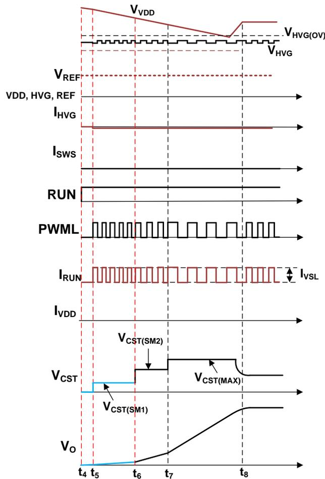
Figure 4. Behavior of Converter at Initial Power Stage
