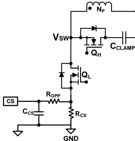
Figure 9. Typical Configuration of the CS Pin
