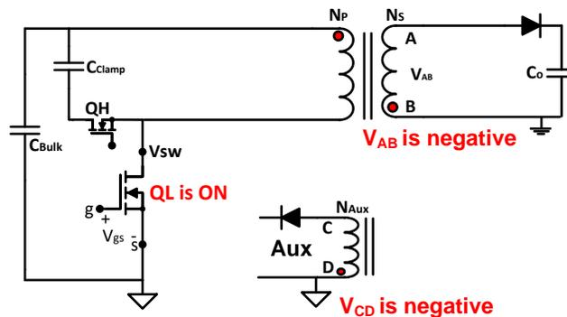
Figure 5. Transformer Test Showing Correct Polarities
