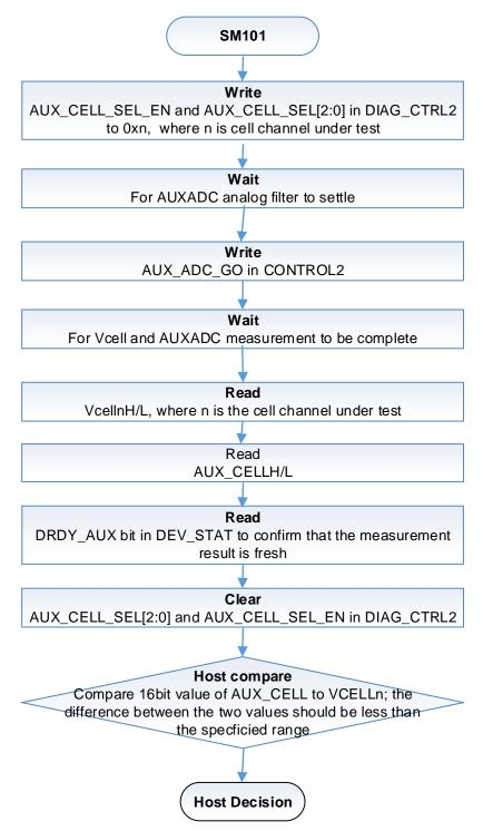
Figure 6. SM101: VCell ADC Path Accuracy Check
