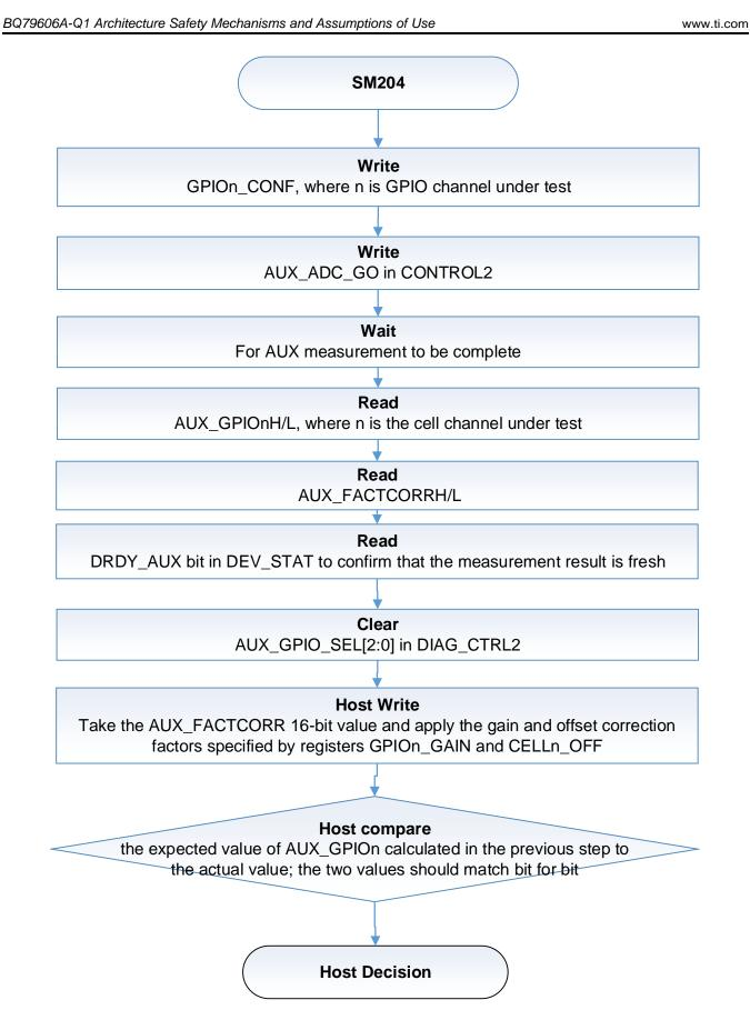
Figure 14. SM204: AUXADC Gain Offset and Output Register Check
