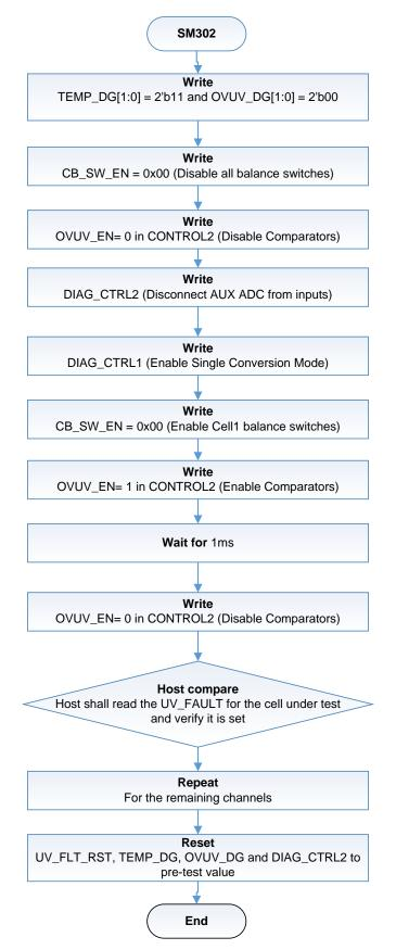
Figure 18. SM302: OV/UV Multiplexor Selector integrity
