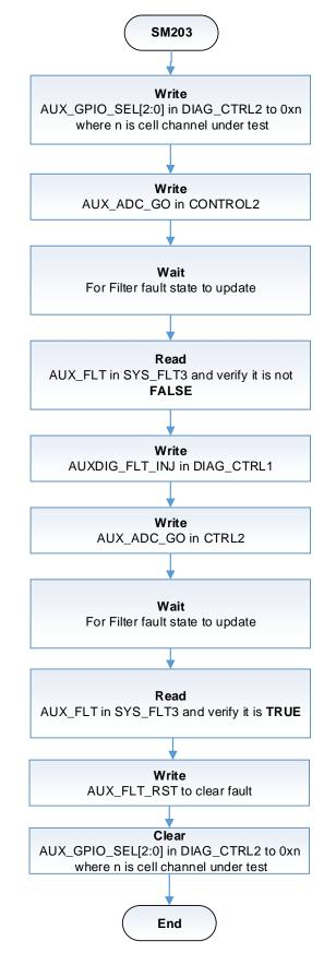
Figure 13. SM203: AUXADC Redundant Digital Filter Fault Injection
