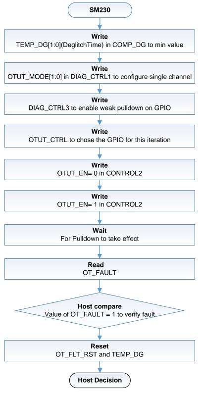
Figure 15. SM230: GPIO Pin Open Check
