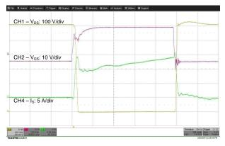
Figure 6. V<sub>DS</sub>, V<sub>GS</sub>, I<sub>S</sub> Switching Cycle
