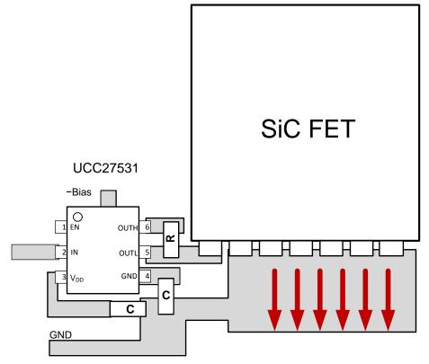
Figure 12. Driver and MOSFET Layout
