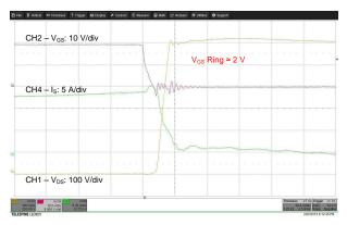
Figure 9. V<sub>DS</sub>, V<sub>GS</sub>, I<sub>S</sub> Turnoff, No Negative Drive
