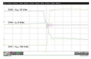
Figure 8.  $V_{DS}$ ,  $V_{GS}$ ,  $I_D$  Turnoff Transition
