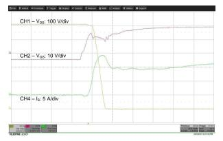
Figure 7. V<sub>DS</sub>, V<sub>GS</sub>, I<sub>S</sub> Turnon Transition
