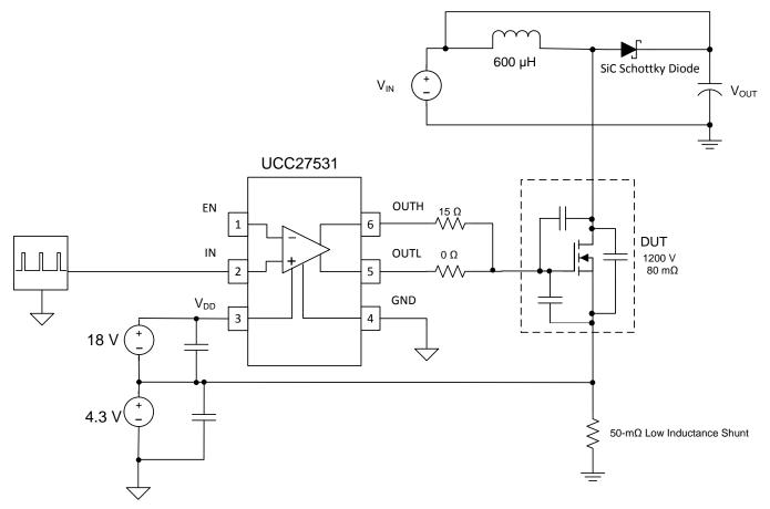
Figure 5. UCC27531 SiC MOSFET Demonstration Circuit Diagram
