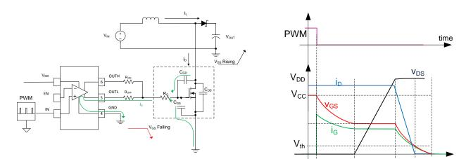
Figure 3. Turnoff Circuit with Parasitic Capacitance
