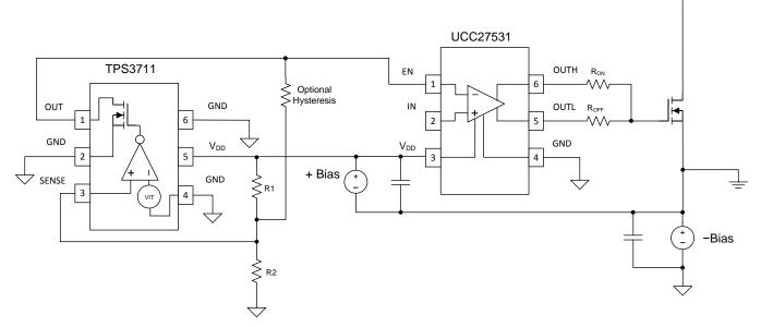
Figure 11. TPS3711 to Program UCC27531 UVLO Thresholds
