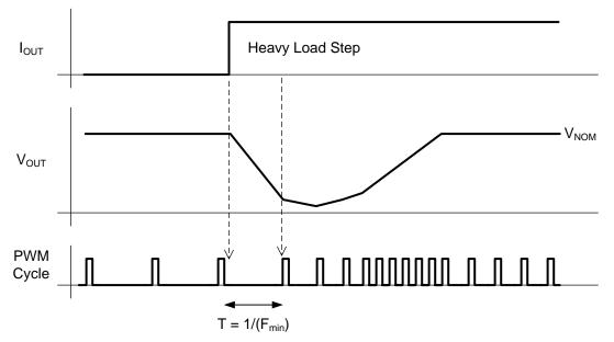
Figure 3. Output Transient Drop at F<sub>min</sub> – When Load Step Occurs just After PWM Cycle
