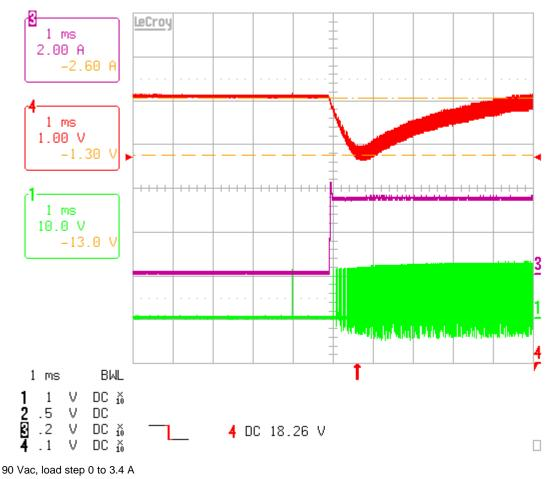
Ch4: V<sub>out</sub>; Ch3: I<sub>load</sub>; Ch1: Gate drive
