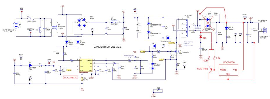
Figure 6. Modification of Standard EVM572 Schematic to Add UCC28633 PSR Controller and UCC24650 Secondary-Side Voltage Monitor and Wake-Up Circuit
