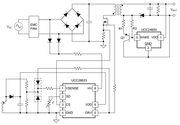
Figure 5. Addition of UCC24650 Secondary-Side Voltage Monitor and Wake-Up Circuit
