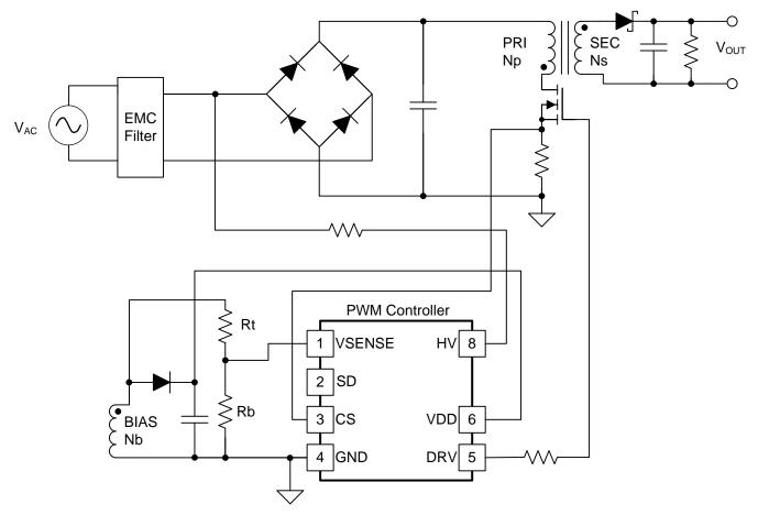
Figure 1. Typical PSR Flyback Power Stage and Controller
