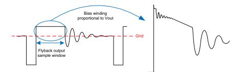
Figure 2. Indirect Output Voltage Sense through Flyback Bias Winding
