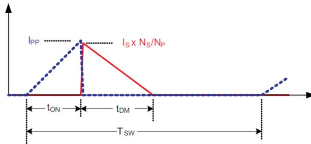
**Figure 3. Transformer Current**
