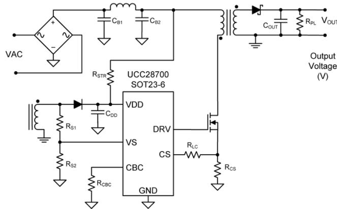
**Figure 1. UCC28700 Application Circuit**
