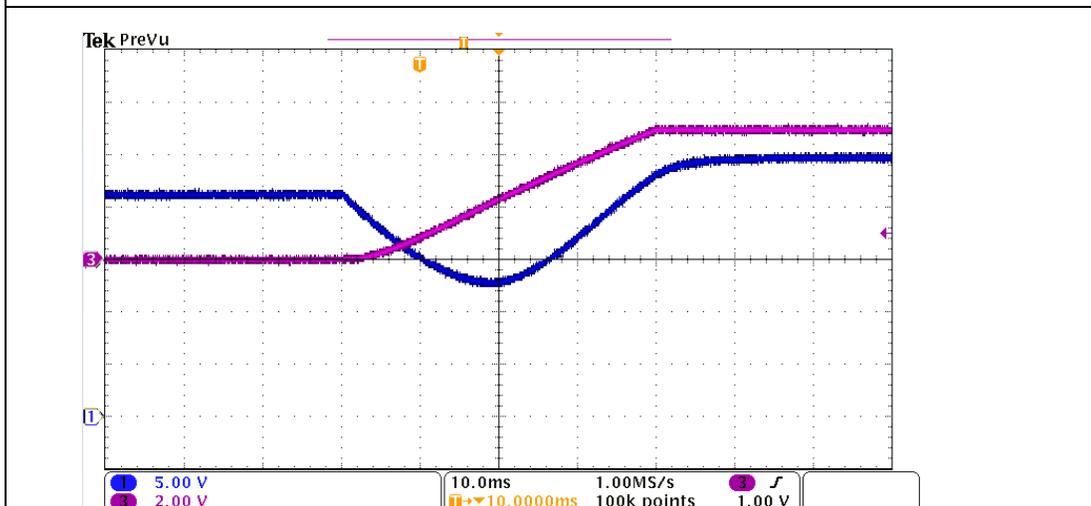
Figure 6. UCC28700 Start-up Waveform with  $C_{DD} = 4.7 \mu\text{F}$ ,  $R_{CS} = 1.8 \Omega$
