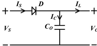
**Figure 2. UCC28700 Secondary Side Circuit**
