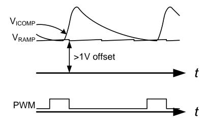
Figure 4. The wide PWM pulses carry enough energy to create audible noise.
