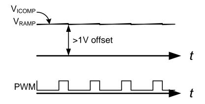
Figure 3. Process variations may result in PWM pulses at no-load.
