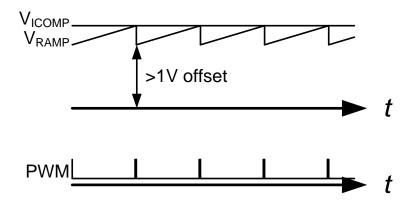
Figure 2. Eventually, during no-load, the falling output voltage will require narrow PWM pulses to maintain regulation, the rising V<sub>RAMP</sub> signal intersects VICOMP and very narrow PWM pulses result.
