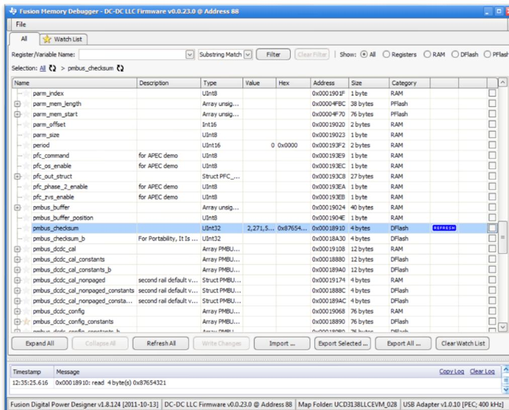
Figure 80. GUI Debugger
