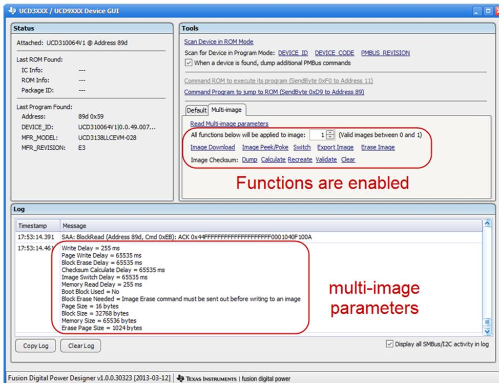
Figure 66. Functions Enabled After Reading Multi-image Parameters
