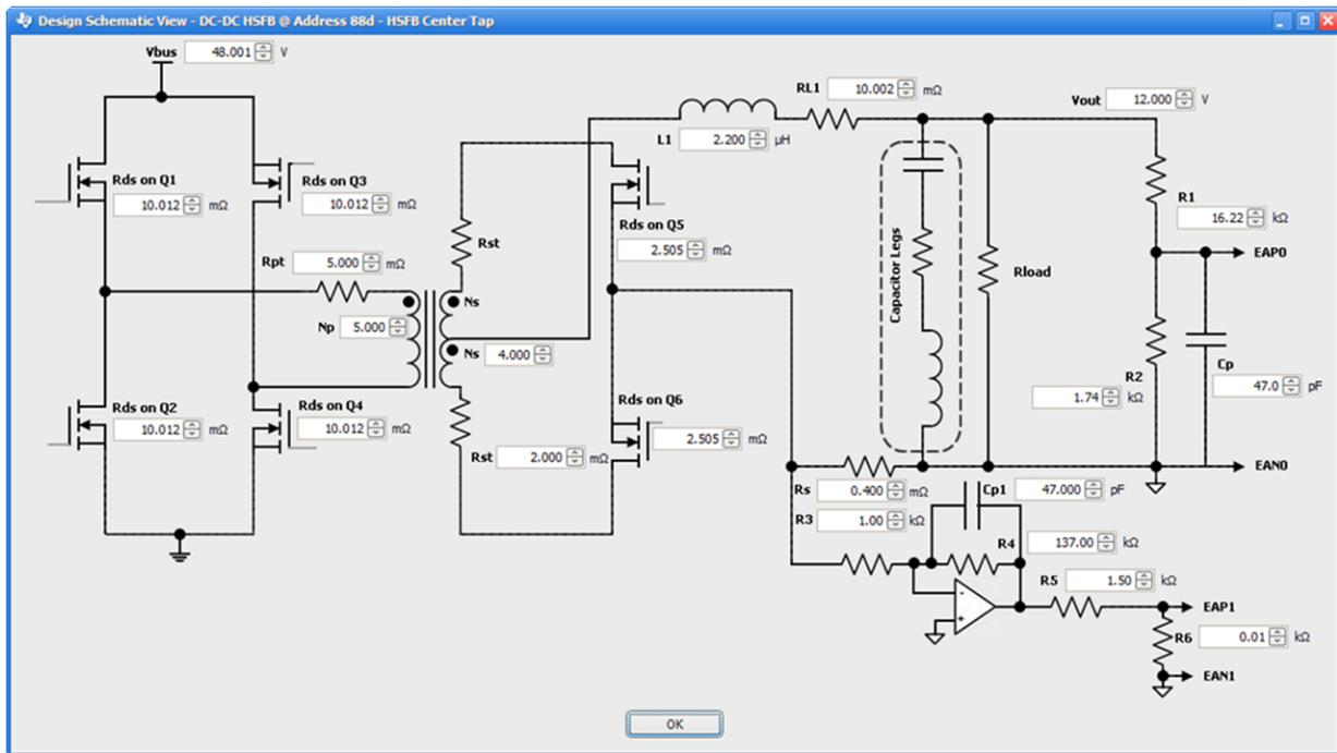
Figure 25. HSF8 Schematic Being Modeled
