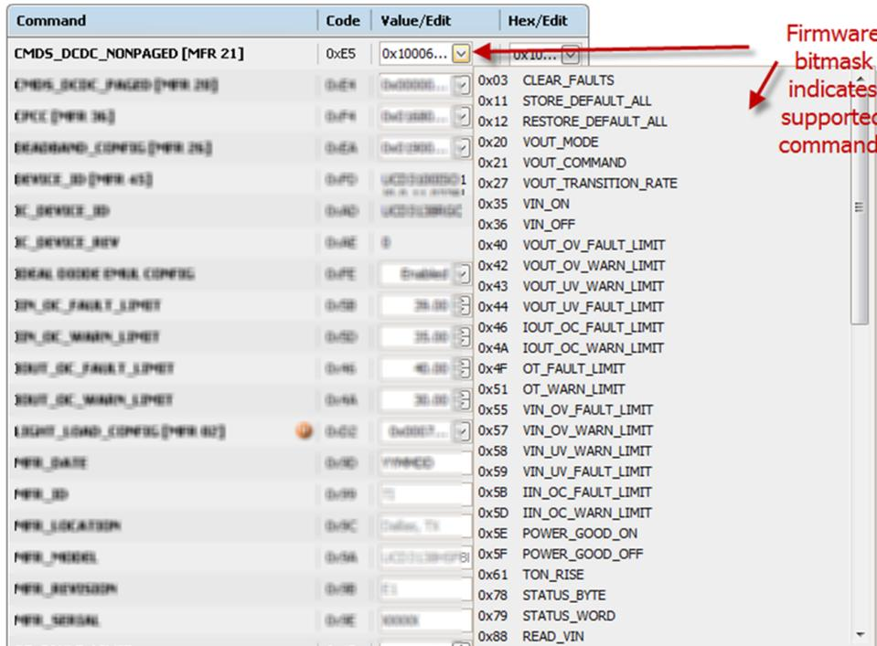
Figure 21. Displays the List of Commands the Firmware Supports
