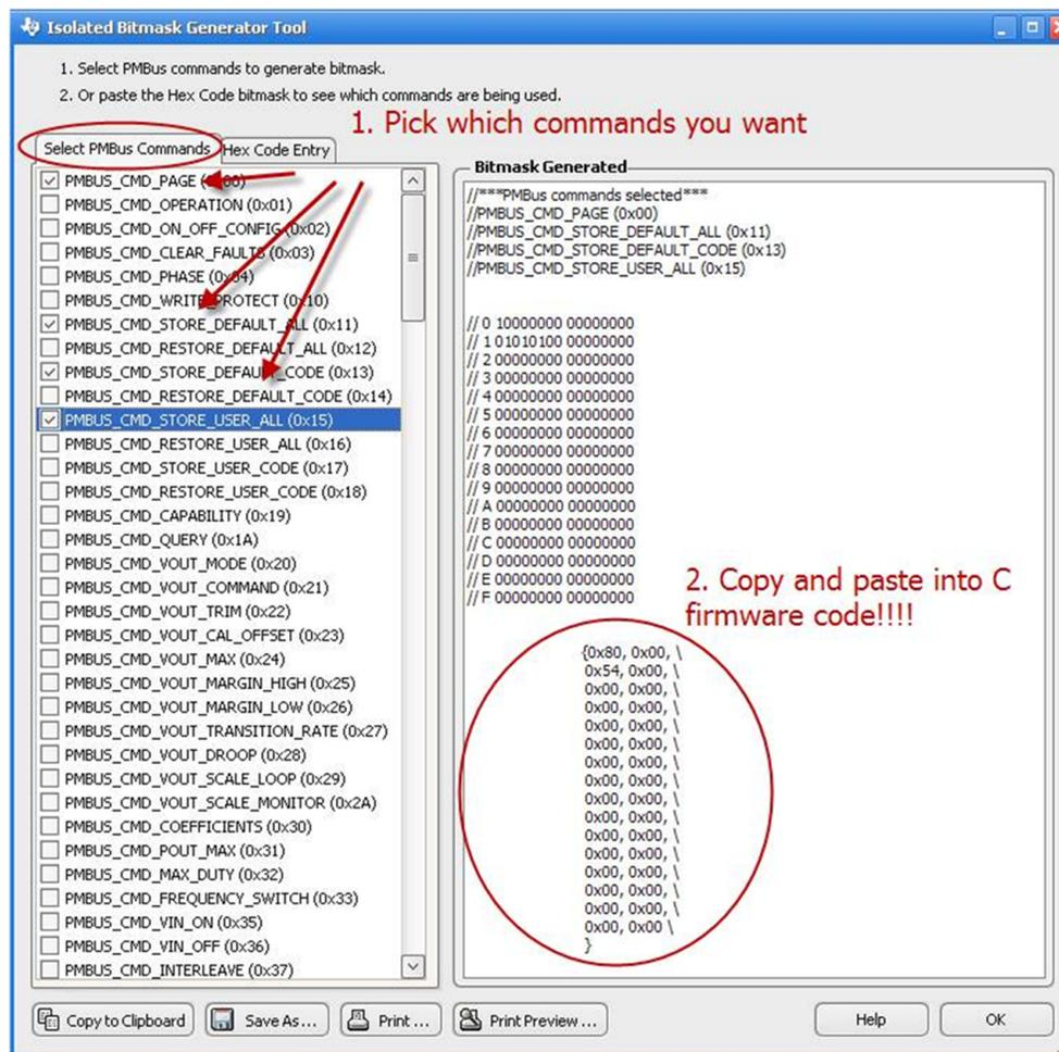
You can also work in reverse by pasting a known bitmask in C code and then see what commands those bitmasks were indicating. You can also go back to the Select PMBus commands tab and all the indicated ones are checked.
