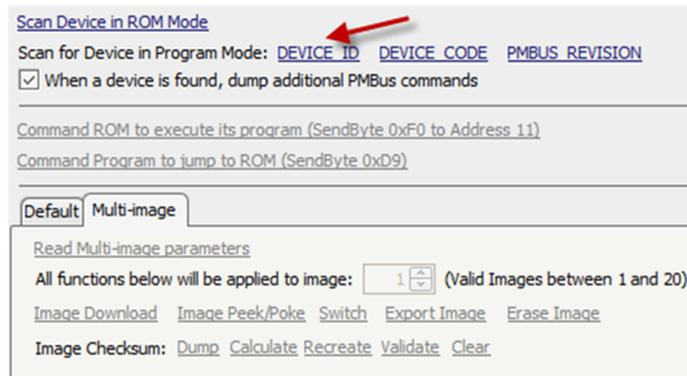
Figure 64. Scan for Device ID to Activate Multi-image
