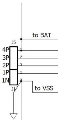
**Figure 3. Lithium-Ion Cell Connections**
