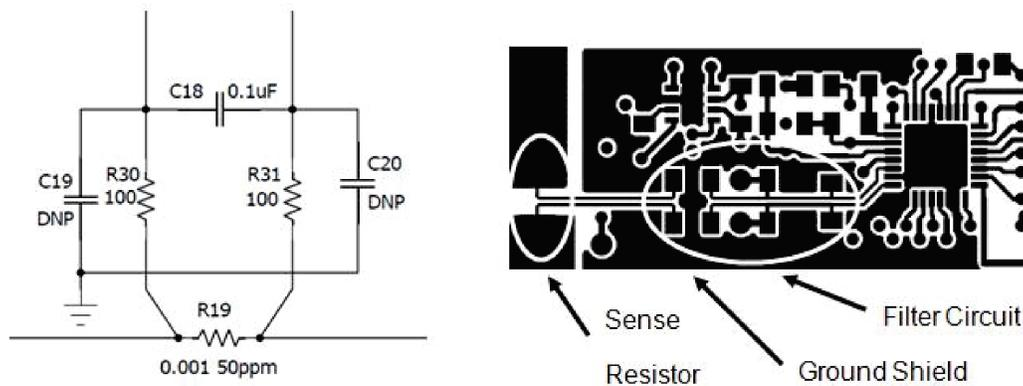
Figure 5. Differential Filter
