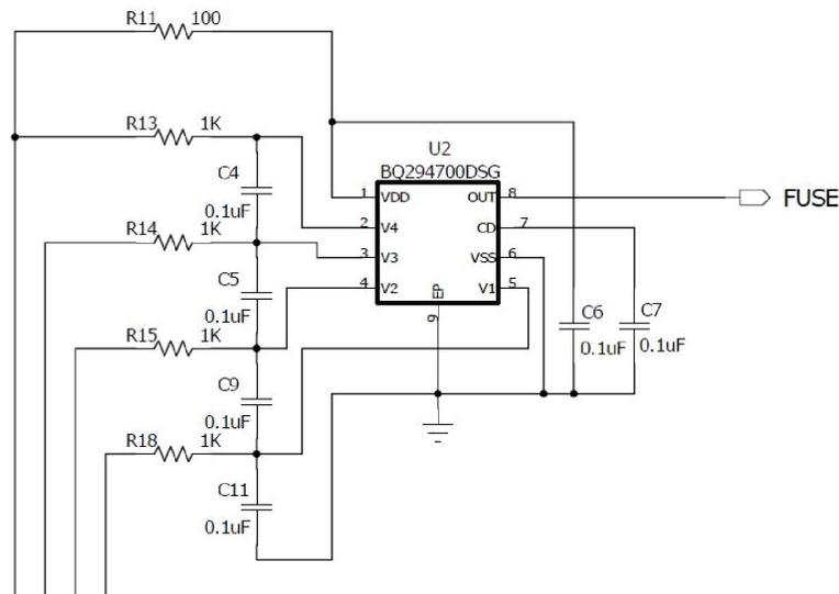
Figure 16. bq294700 Cell Inputs and Time-Delay Capacitor
