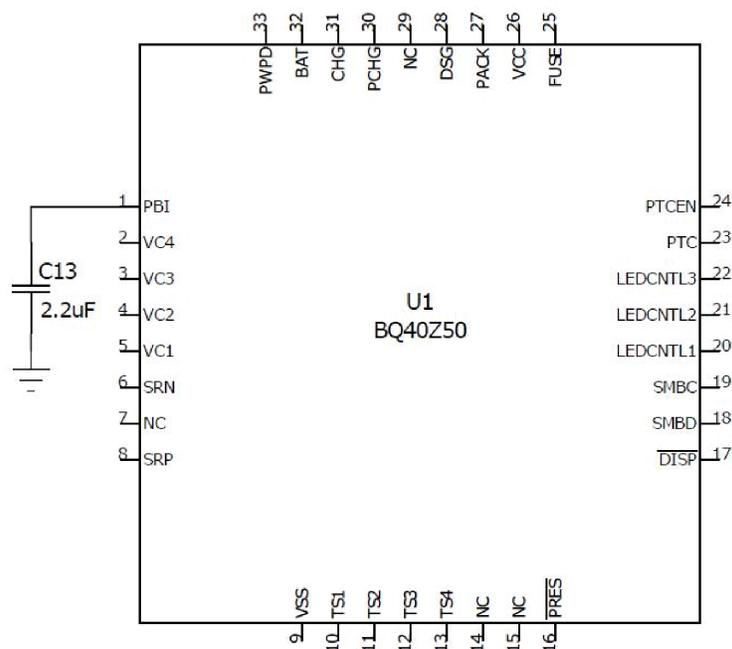
Figure 6. Power Supply Decoupling
