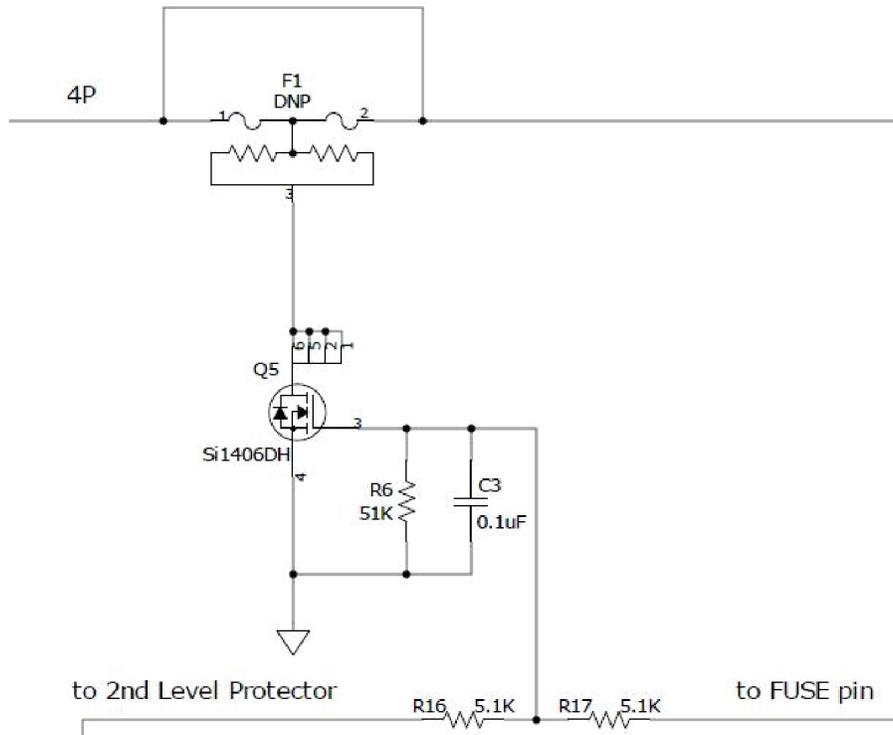
Figure 2. FUSE Circuit
