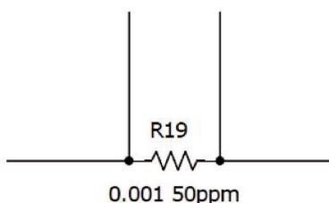
**Figure 4. Sense Resistor**
