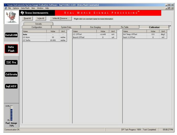
Figure 2. bq274xx EVSW Calibration Data Flash Screen
