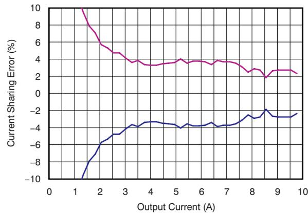
Figure 3. Load Share Error Result for Two Rails
