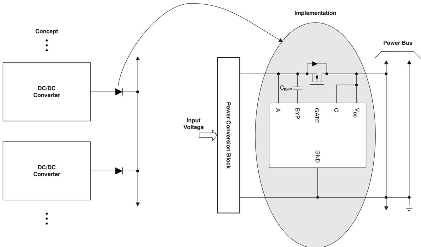
**Figure 1. Redundant System Using TPS2412 OR-ing FET Controller**
