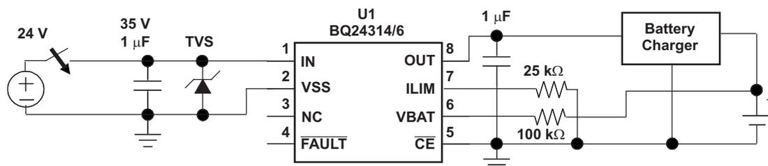
Figure 1. 24-V Hot Plug-in Transient Test Schematic
