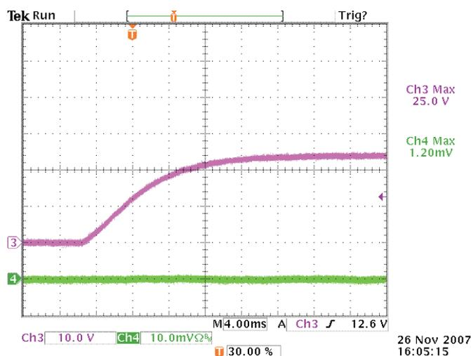
Figure 2. Soft Start-up of 24-V Input Voltage, CH3 10 V/div, CH4 5 A/div
