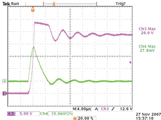
Figure 5. 24-V Hot Plug-in With TVS Zener Diode DFLT24A, CH3 5 V/div, CH4 5 A/div
