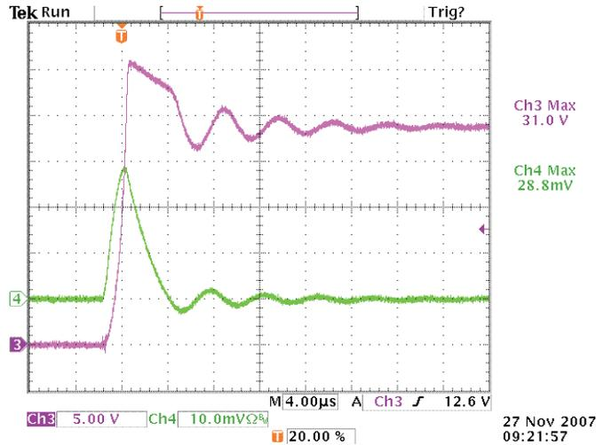
Figure 4. 24V Hot Plug-in With TVS Zener Diode MMBZ27VCLT, CH3 5V/div, CH4 5A/div
