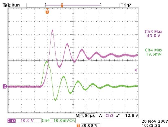
Figure 3. 24-V Hot Plug-in Without TVS Zener Diode, CH3 10 V/div, CH4 5 A/div
