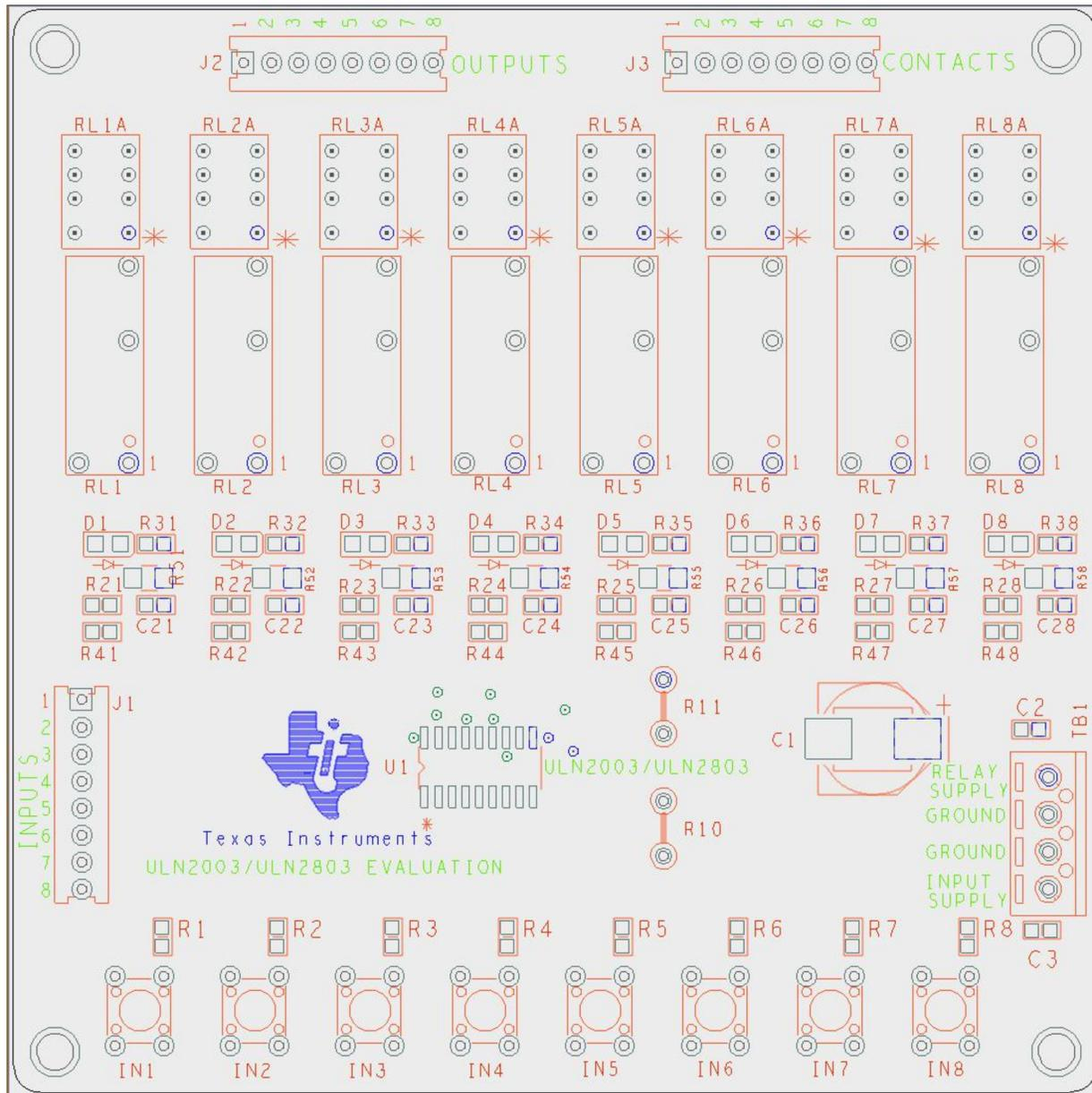
Figure 1. Physical Structure for the ULN2003EVM (Approximate Layout)
