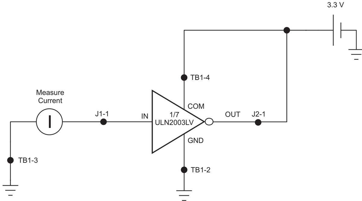
**Figure 8.  $I_{(off)}$  Schematic**
