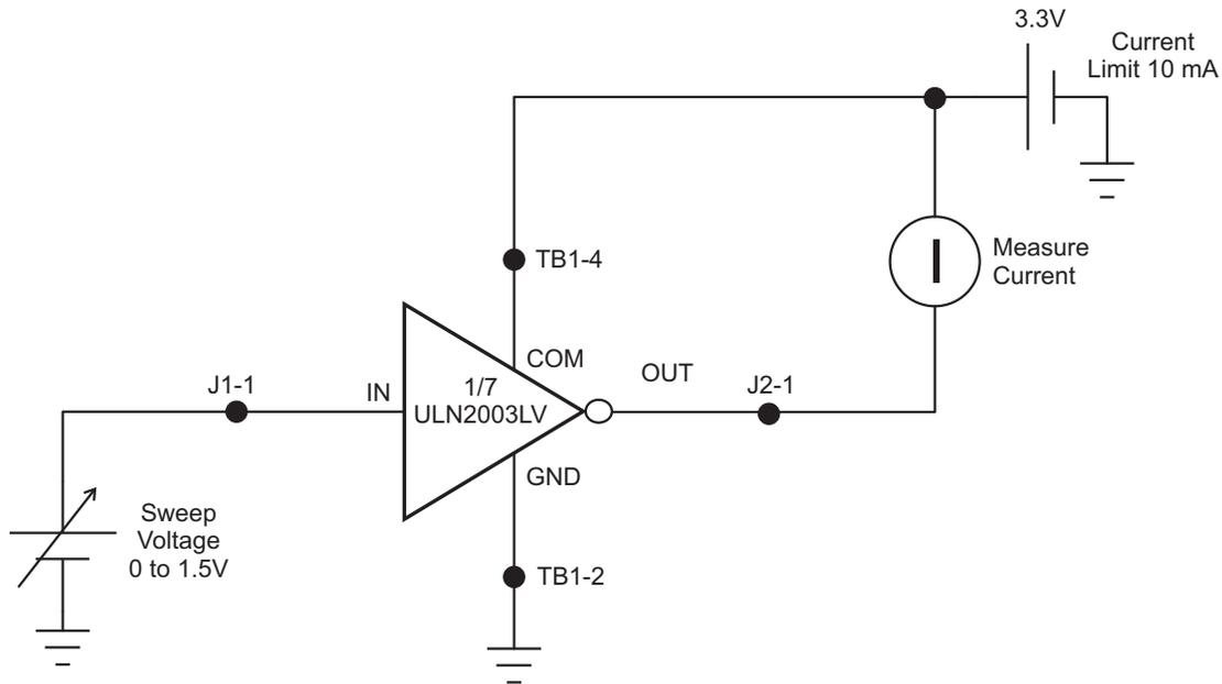
Figure 4.  $V_I(\text{on})$  and  $V_I(\text{off})$  Schematic
