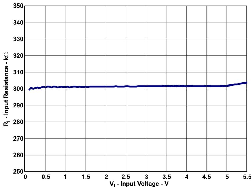
Figure 21.  $R_{IN} = V_{IN}/I_{IN}$  vs  $V_{IN}$
