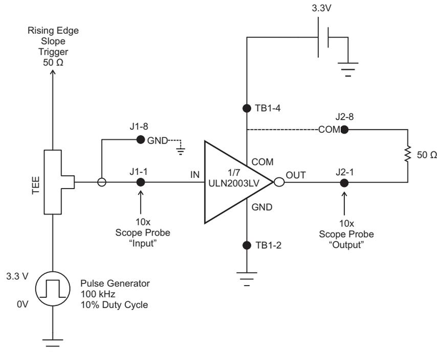
Figure 13.  $T_{PHL}$  Schematic
