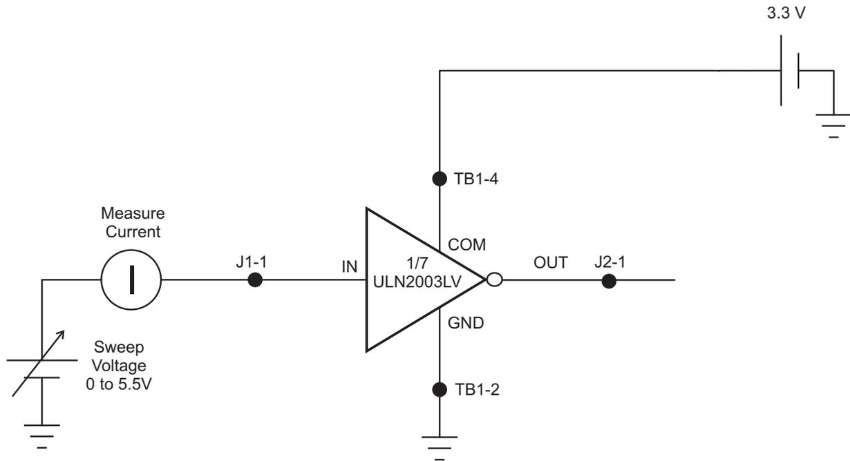
Figure 6.  $I_{(on)}$  Schematic
