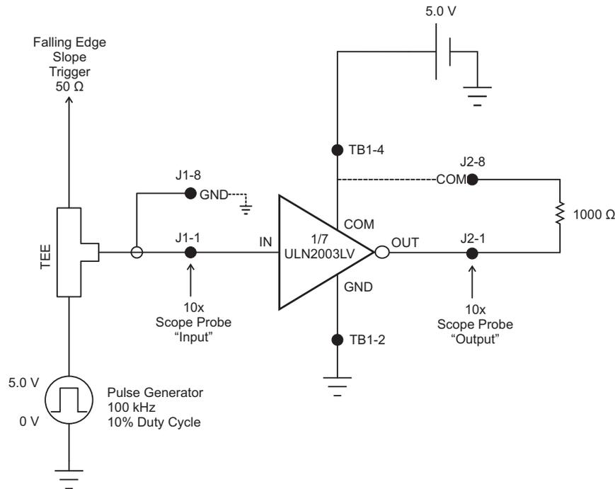
Figure 19.  $T_{PLH}$  Schematic
