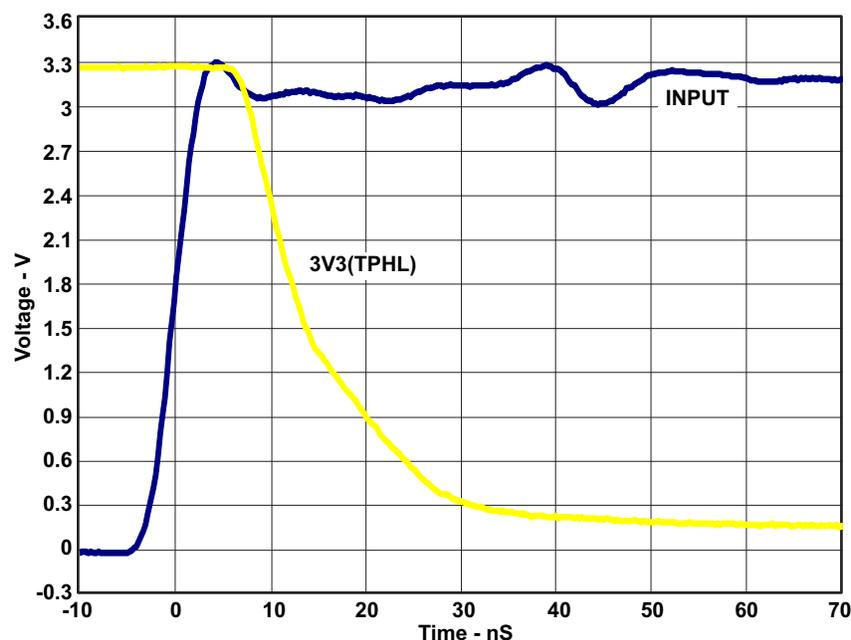
Figure 14.  $T_{PHL}$  3.3V 50Ω pullup = 13nS
