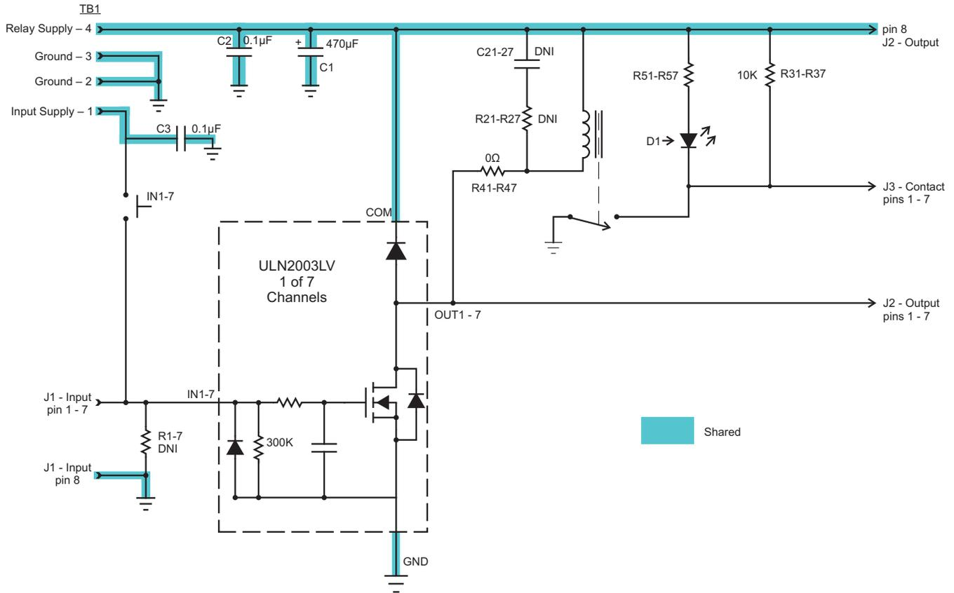
**Figure 3. Single Channel Schematic**
