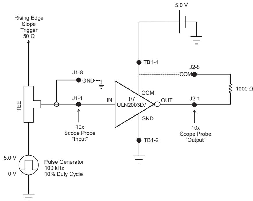
Figure 17.  $T_{PHL}$  Schematic
