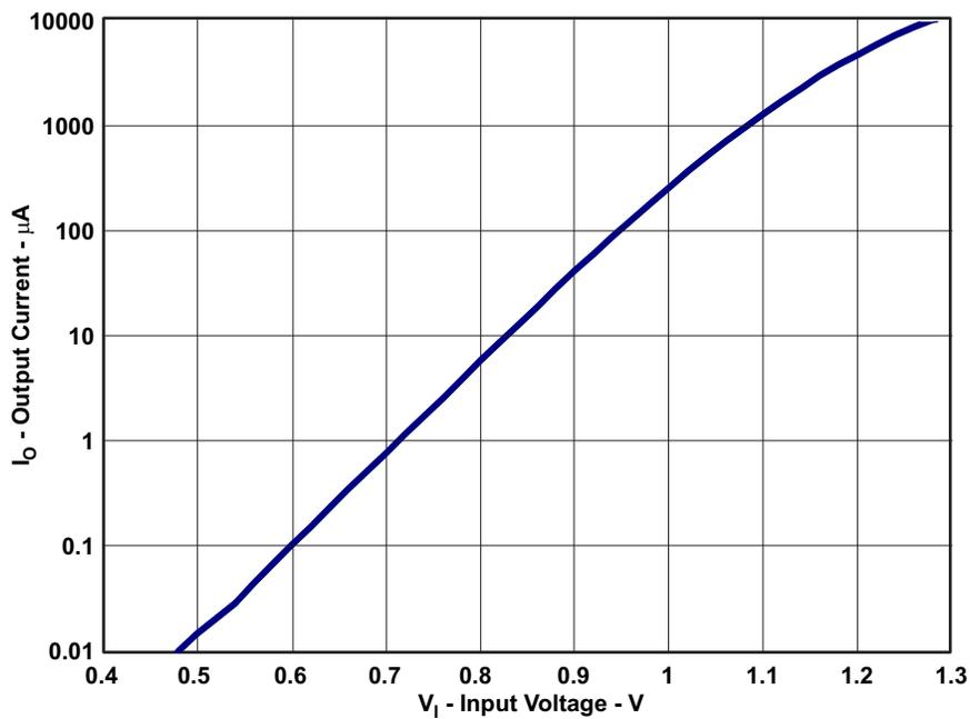
Figure 5.  $V_I(\text{on, off}) = I_{OS}(3.3V)$  vs  $V_{in}$
