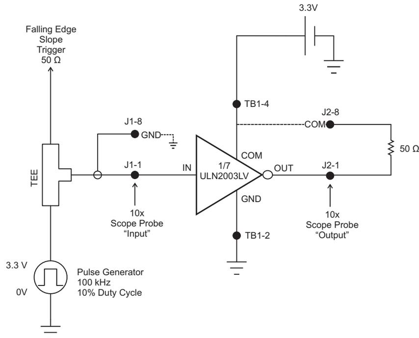
Figure 15.  $T_{PLH}$  Schematic
