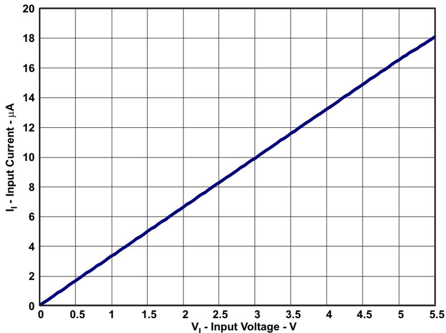
Figure 7.  $I_{(on)} = I_{IN}$  vs  $V_{IN}$
