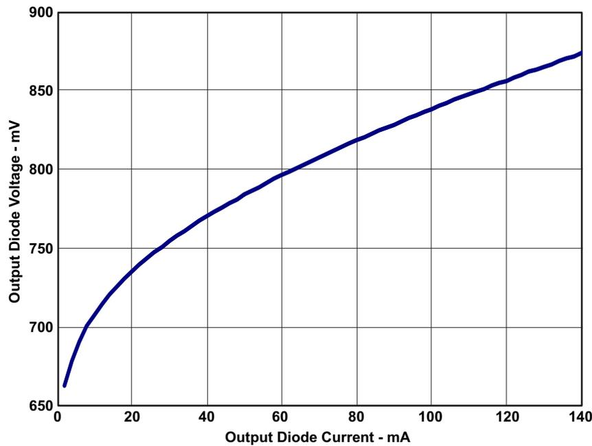
Figure 23. VF = Diode(V) vs Diode(I)
