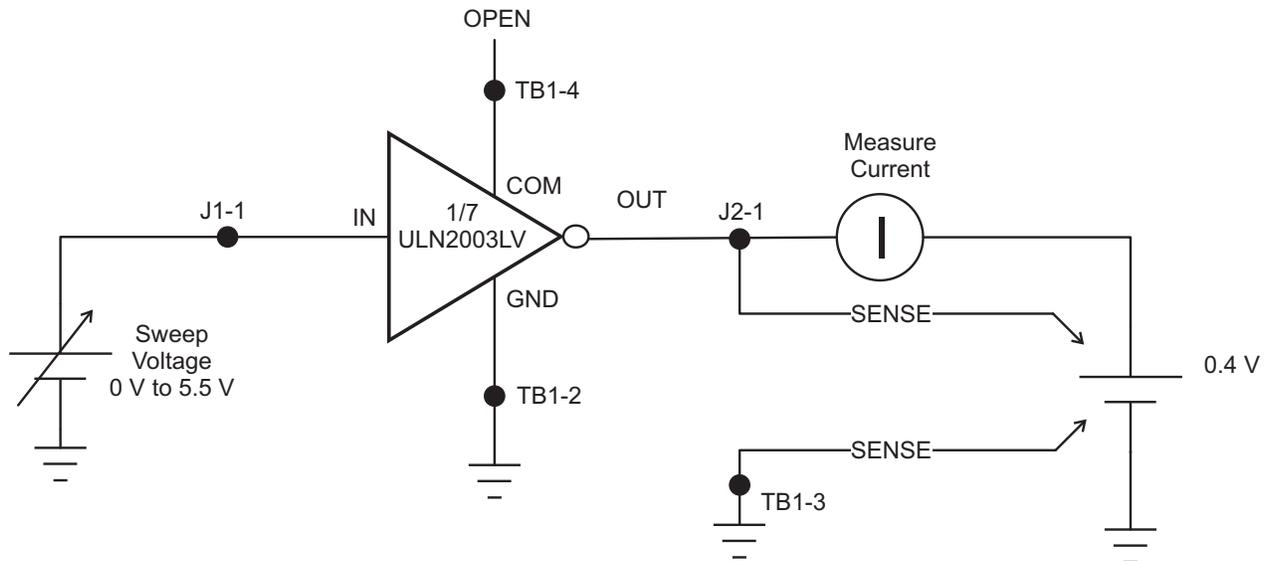
Figure 11.  $I_{OUT(on)}$  Schematic
