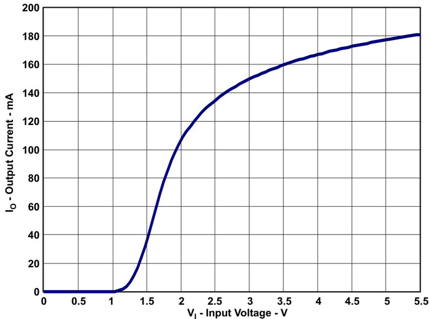
Figure 12.  $I_{OUT(on)} = I_{OS(400mV)}$  vs  $V_{IN}$
