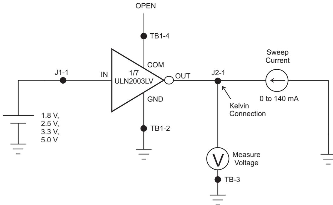
Figure 9. VOL Schematic
