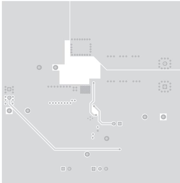
**Figure 15. CSD87355Q5DEVM-820 Internal Copper Layer 1 (X-Ray Top View)**
