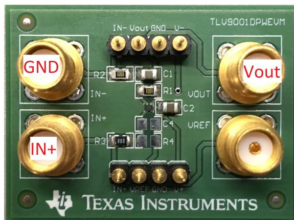
Figure 6. Non-Inverting Amplifier Configured on TLV9001DPW EVM
