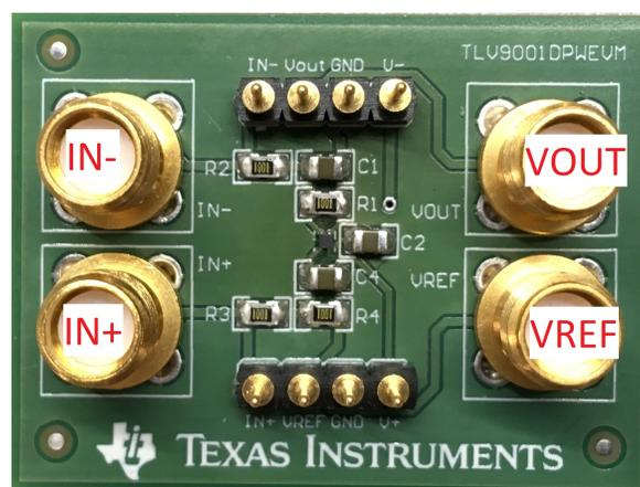
Figure 4. Difference Amplifier Configured on TLV9001DPW EVM
