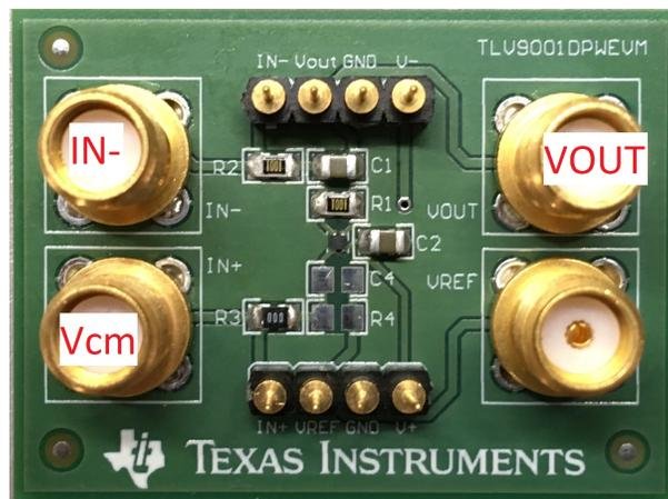
**Figure 8. Inverting Amplifier Configured on TLV9001DPW EVM**
