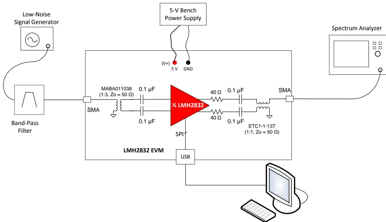
Figure 2. LMH2832 Evaluation Board Setup Block Diagram
