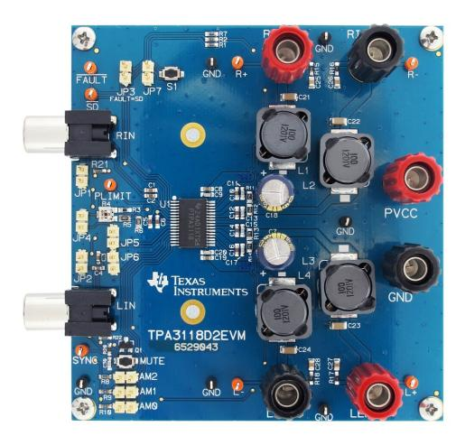
Figure 1. TPA3118D2EVM Photo, Top View
