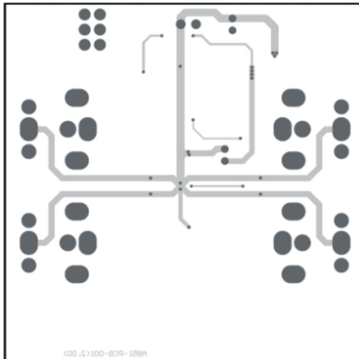
Figure 16. DRV602EVM2 PCB Bottom Layer
