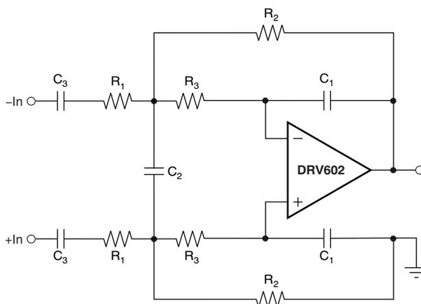
**Figure 4. Differential Input, Second-Order Active Low-Pass Filter**
