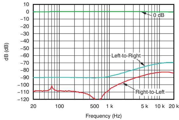
**Figure 8. Channel Separation**
