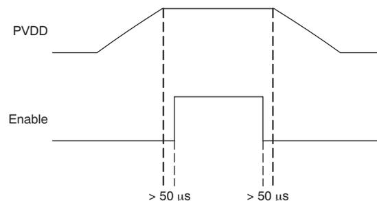
**Figure 2. Power-Up/-Down Sequence**
