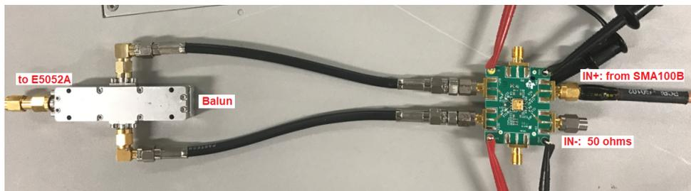
Figure 6. SMA100B + LMH5401-SP Phase Noise Setup
