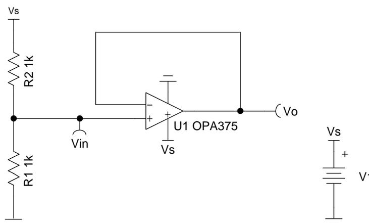
In the first example, the positive supply voltage is 5 V, which sets the DC input voltage ( $V_{in}$ ) to 2.5 V. Solving Equation 2 for the OPA375 with a 5-V positive supply once again yields Equation 3. The 2.5-V DC input satisfies this inequality, so the output will not clip. Figure 5 shows the transient simulation that supports this conclusion. Notice that  $V_{in}$  exactly matches  $V_o$ , both of which are 2.5-V DC. In this case, non-RRI amplifiers will work as well as RRI amplifiers.
