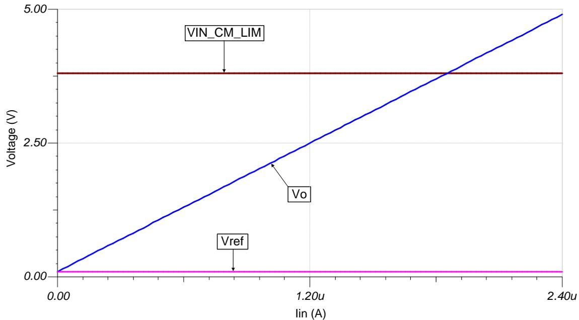
The input common-mode voltage for a transimpedance amplifier is set by  $V_{ref}$ , the voltage at the positive input. This voltage is almost always either connected to ground or set to a very small offset voltage, so RRI amplifiers are almost never required. This concept is summarized in [Equation 13](#).
