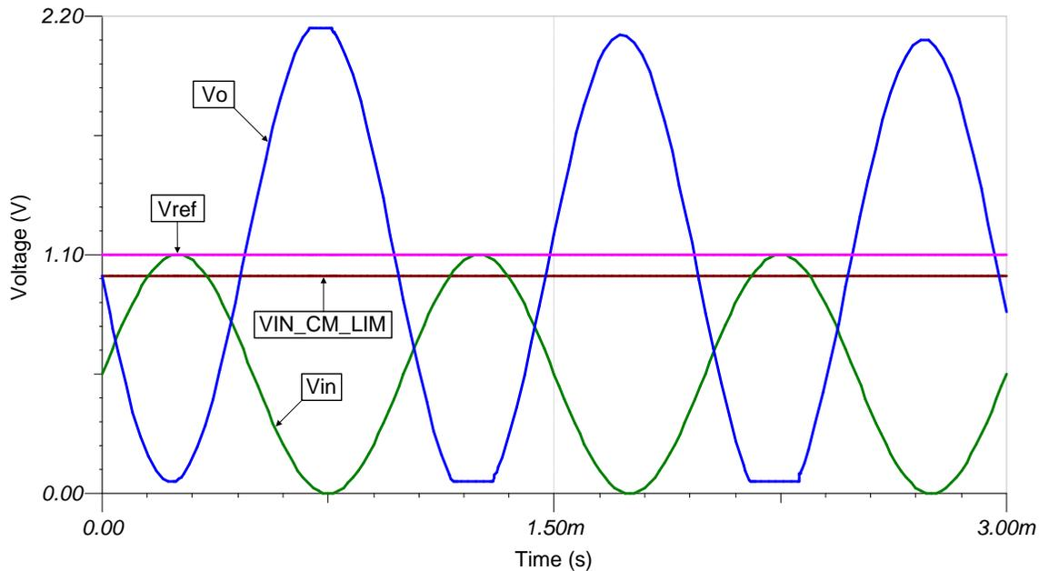
As long as Equation 11 is satisfied, RRI amplifiers are not needed for basic inverting amplifier circuits. This inequality is a simplified version of the equations used previously in this section and assumes that  $V_{ref}$  (the voltage at the positive input) is set to mid-rail. For inverting amplifiers with the positive input tied to ground, RRI amplifiers are never needed. Both the previous statement and Equation 11 also apply to AC coupled inverting amplifiers.
