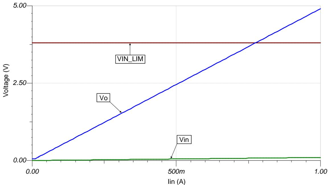
Like the transimpedance amplifier, an RRI amplifier is almost never required for a low-side current sensing circuit. This is due to the very low input voltage, which is equivalent to the input common-mode voltage. As long as is satisfied, RRI amplifiers are not needed.
