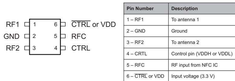
**Figure 4. PE42359 RF Switch Pin Configuration and Description**
