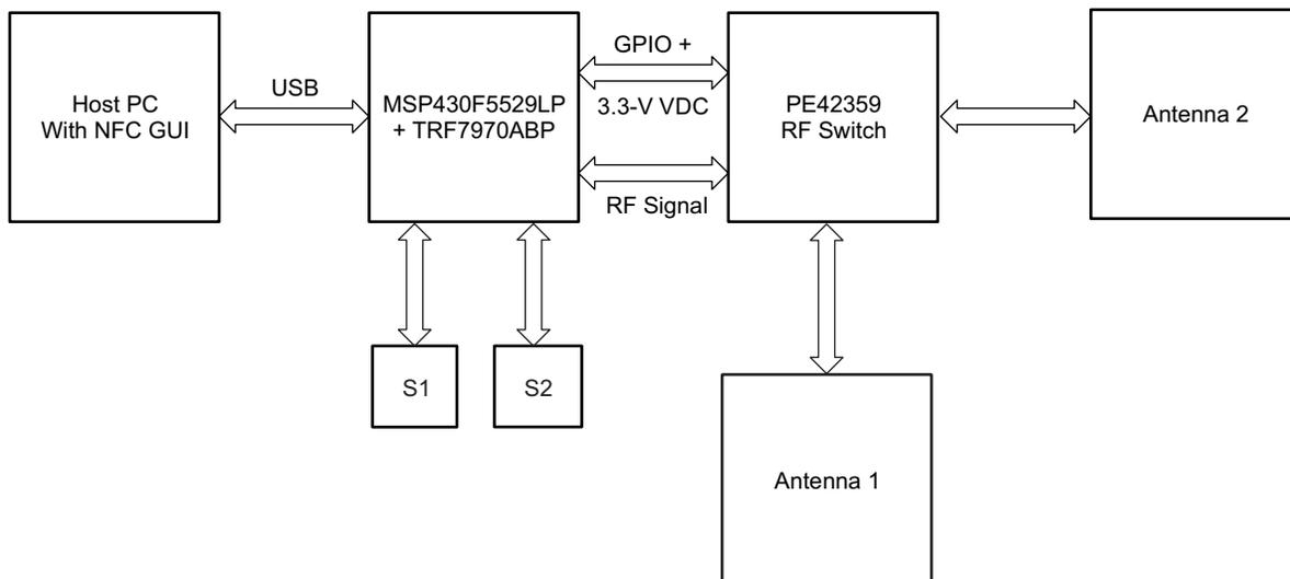
**Figure 1. Block Diagram of Reader Antenna Multiplexing Demo**
