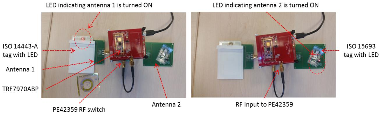
Figure 9. Prototype of TRF7970ABP + PE42359 RF Switch Demonstration
