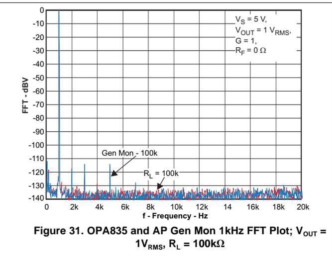
Figure 31. OPA835 and AP Gen Mon 1kHz FFT Plot;  $V_{OUT} = 1V_{RMS}$ ,  $R_L = 100k\Omega$
