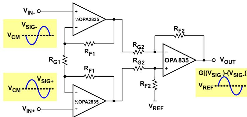
Figure 7. Instrumentation Amplifier
