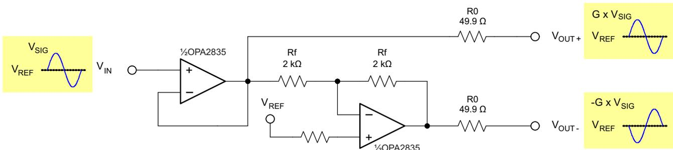
Figure 4. CAT 5 Line Driver with Gain = 2 V/V (6 dB)
