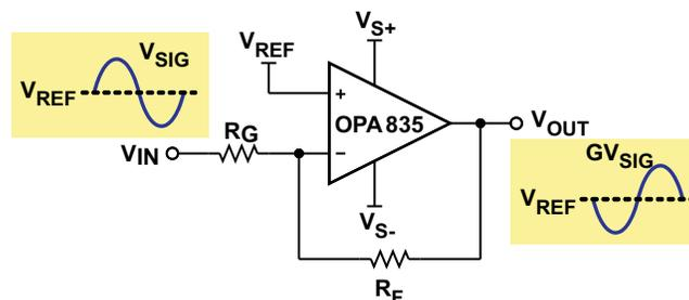
Figure 2. Inverting Amplifier
