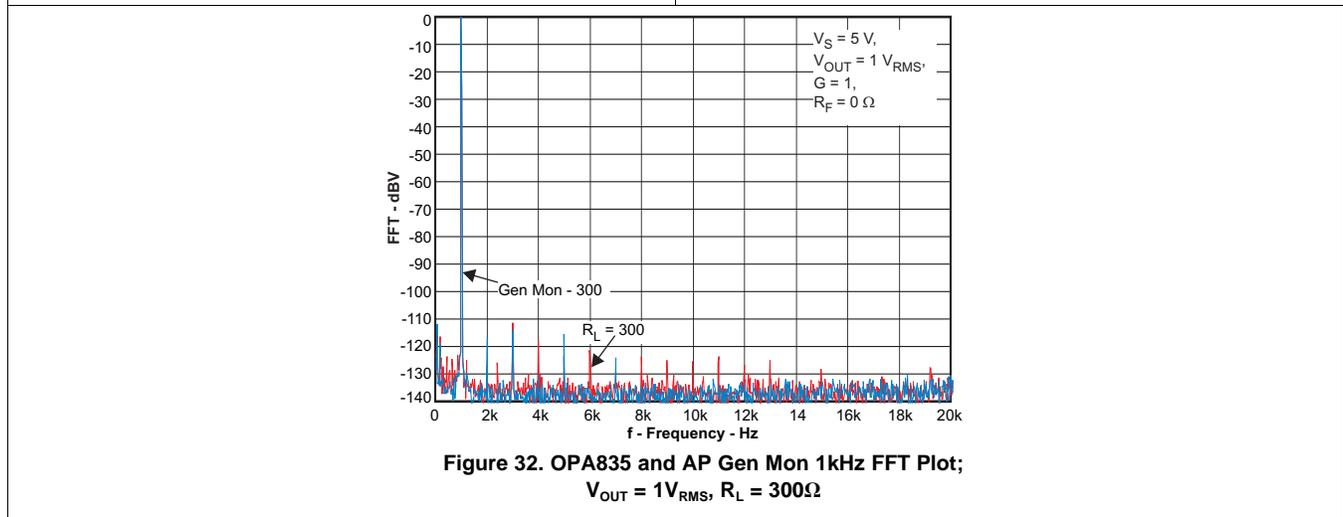
Figure 32. OPA835 and AP Gen Mon 1kHz FFT Plot;  $V_{OUT} = 1V_{RMS}$ ,  $R_L = 300\Omega$
