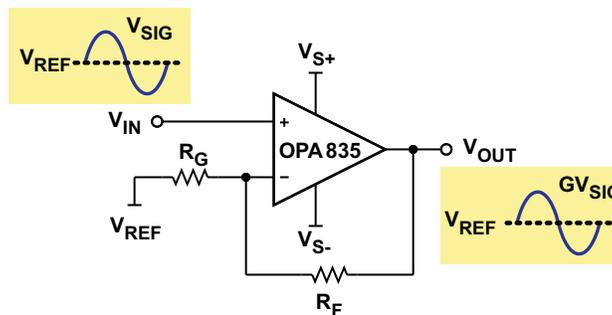
Figure 1. Non-Inverting Amplifier
