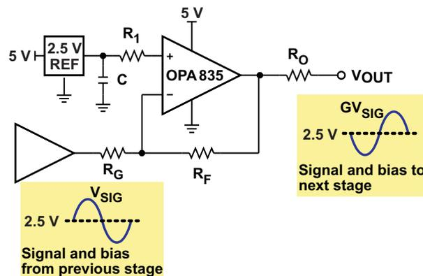
**Figure 17. Inverting Single Supply with Reference**
