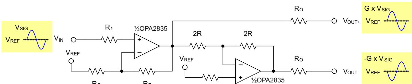
Figure 3. Single Ended to Differential Amplifier
