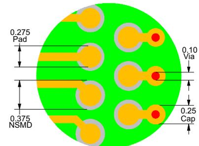
**Figure 7. Example Inner Row Via Escapes to Layer 2**
