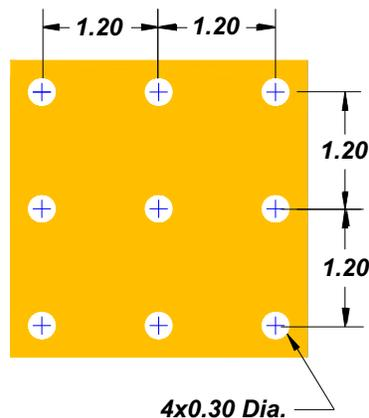
**Figure 8. Example Via Layout Design Via layout – Designs will vary depending on layout constraints**
