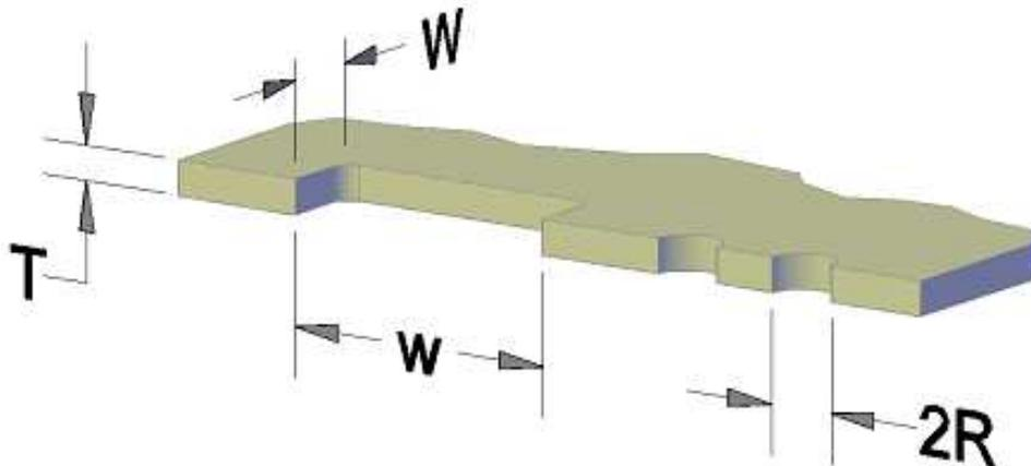
Basic concept: Aspect ratio ( $W/T, 2R/T$ ) > 1.4, Area Ratio ( $W/4T, R/2T$ ) > 66%.
