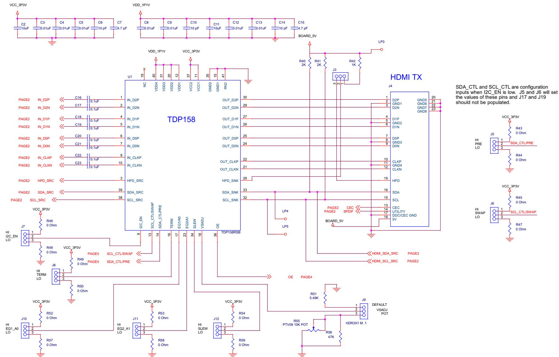
SDA\_CTL and SCL\_CTL are configuration inputs when I2C\_EN is low. J5 and J6 will set the values of these pins and J17 and J19 should not be populated.
