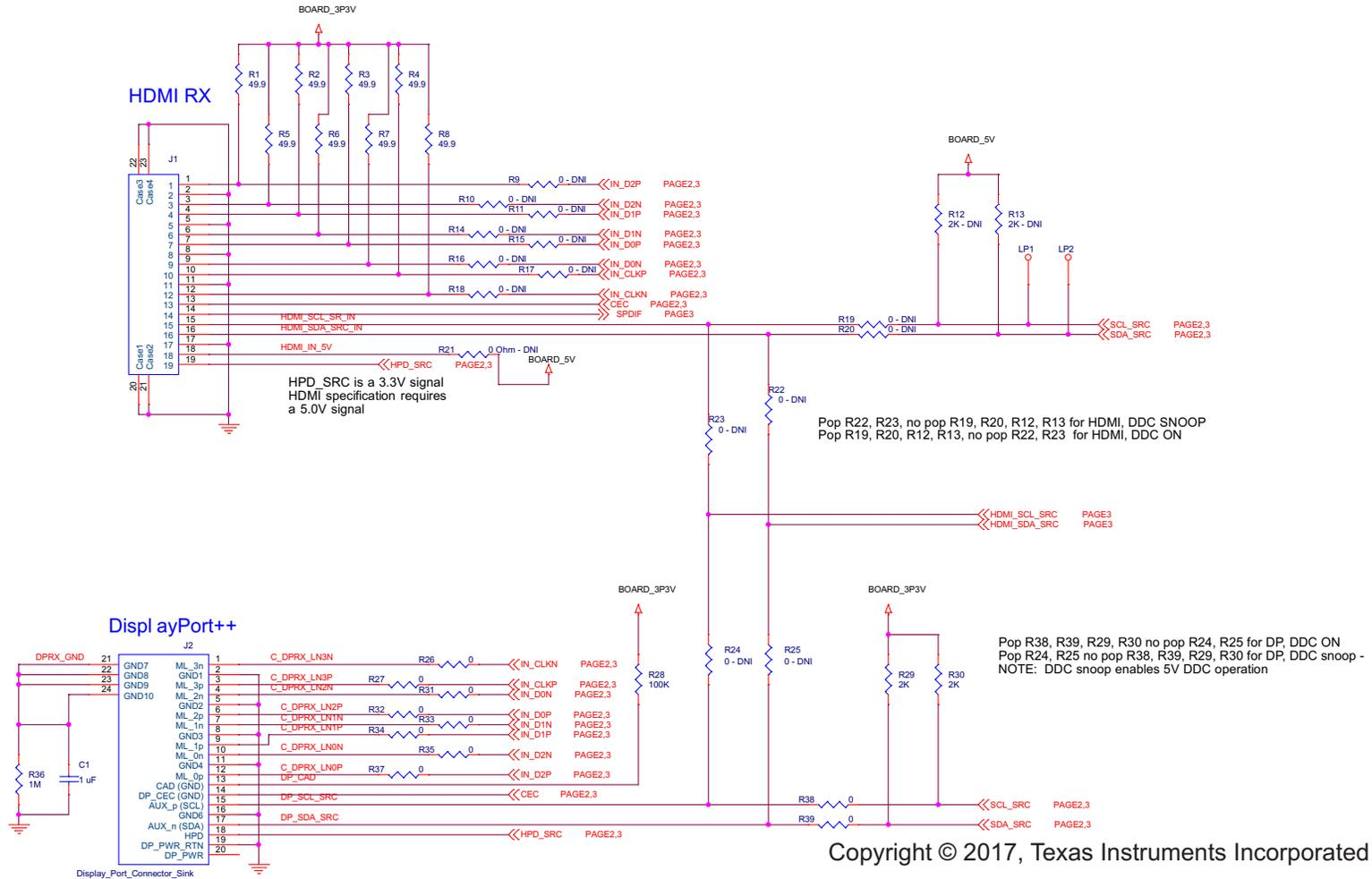
Figure 3. TDP158RSBEVM Schematics (1 of 4) - Input Connectors
