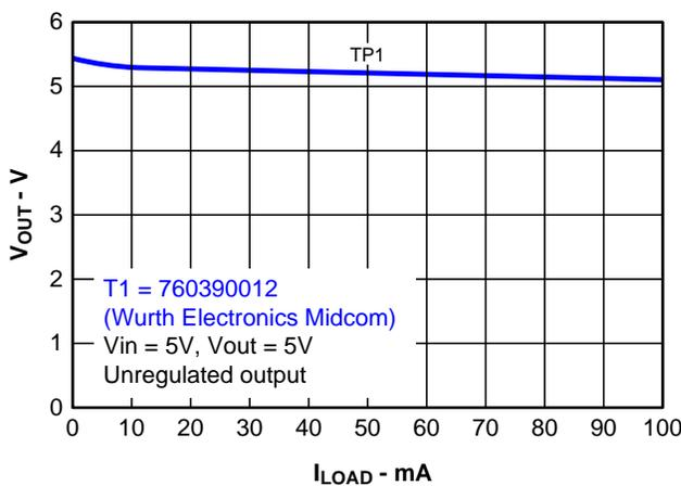
Figure 8. Output Voltage Versus Load Current
