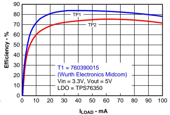
**Figure 13. Efficiency Versus Load Current**
