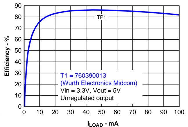
Figure 11. Efficiency Versus Load Current
