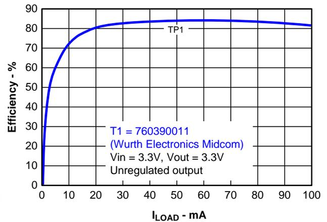
Figure 7. Efficiency Versus Load Current
