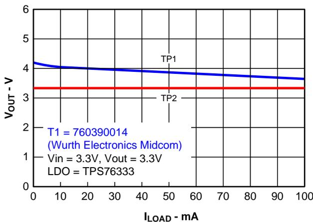
**Figure 14. Output Voltage Versus Load Current**
