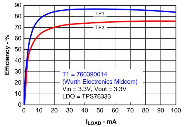
**Figure 15. Efficiency Versus Load Current**
