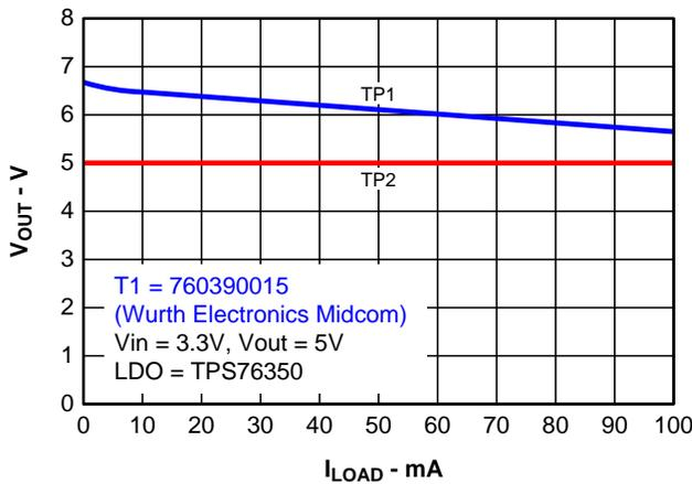
**Figure 12. Output Voltage Versus Load Current**
