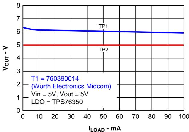
**Figure 16. Output Voltage Versus Load Current**
