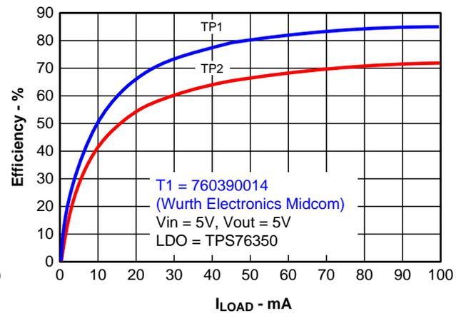
**Figure 17. Efficiency Versus Load Current**
