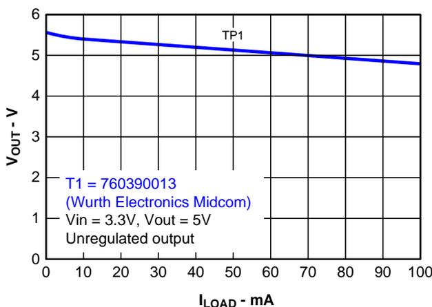
Figure 10. Output Voltage Versus Load Current
