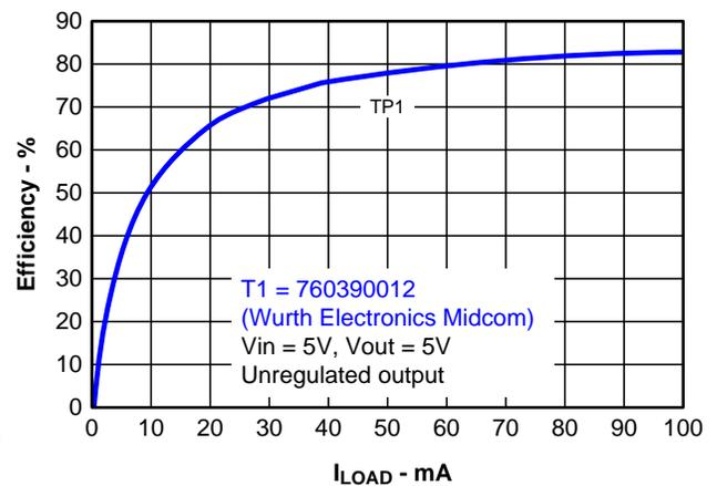
Figure 9. Efficiency Versus Load Current
