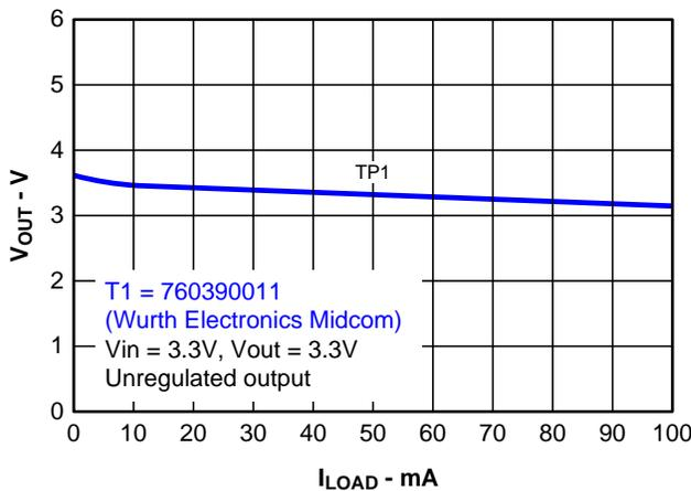
Figure 6. Output Voltage Versus Load Current
