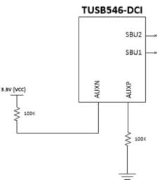
Figure 4. AUXP/N Connections When AUX Bypassed
