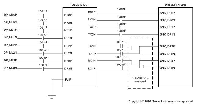
Figure 3. TX1 and RX1 Polarity Swap (FLIP = 0)
