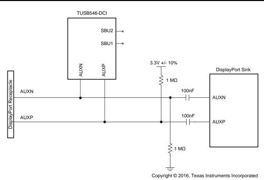
Figure 5. AUX Implementation in DisplayPort Sink Application
