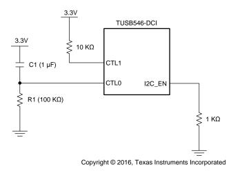
Figure 2. Method to Enable DisplayPort Mode When in GPIO Mode
