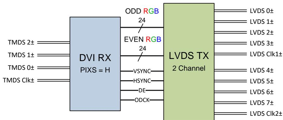
**Figure 2. DVI Receiver to a 2-channel LVDS/OLDI Transmitter**
