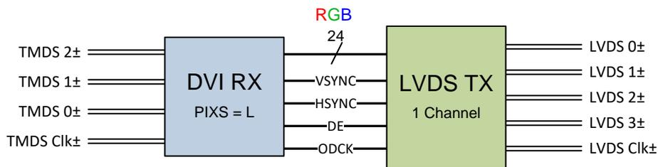
**Figure 1. DVI Receiver to a 1-channel LVDS/OLDI Transmitter**
