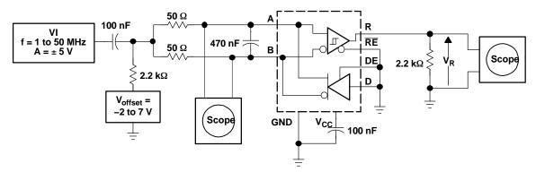
Figure 11. Common-Mode Rejection Test Circuit
