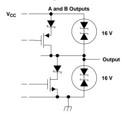
Figure 13. Equivalent Output Schematic of SN65HVD1176
