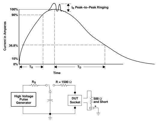
Figure 12. HBM Waveform Description and Simulator
