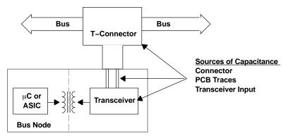
Figure 9. Total Node Capacitance
