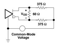
Figure 3. V<sub>OD</sub> Test Over a Common-Mode Load
