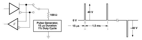
Figure 14. Transient Overvoltage Test of the SN65HVD1176
