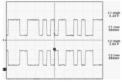
Figure 8. A (CH1) and B (CH2) Outputs With a 0-V Common-Mode Voltage Load
