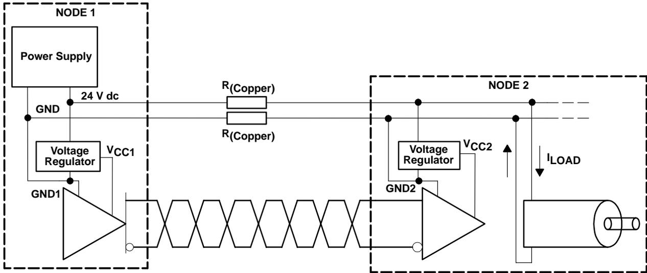
**Figure 6. System With Ground Potential Shift**
