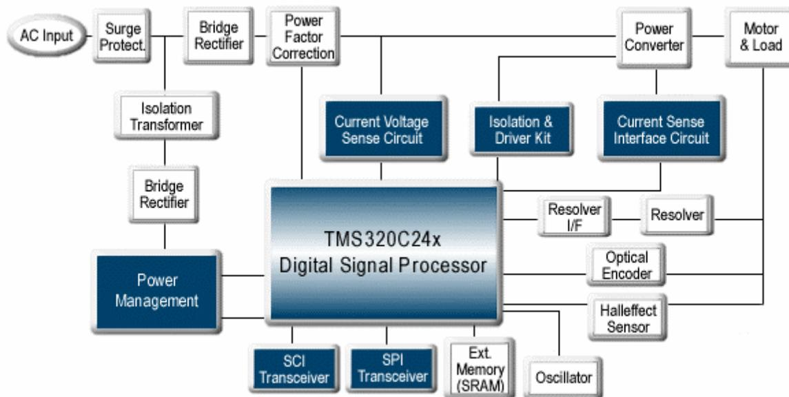
**Figure 1. Digital Motor Control Block Diagram Showing Components Offered by Texas Instruments**
