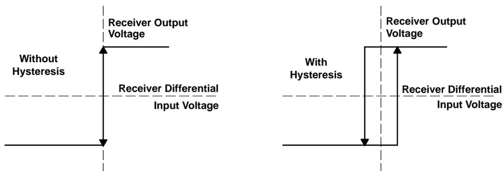
**Figure 4. Receiver Function With and Without Hysteresis**
