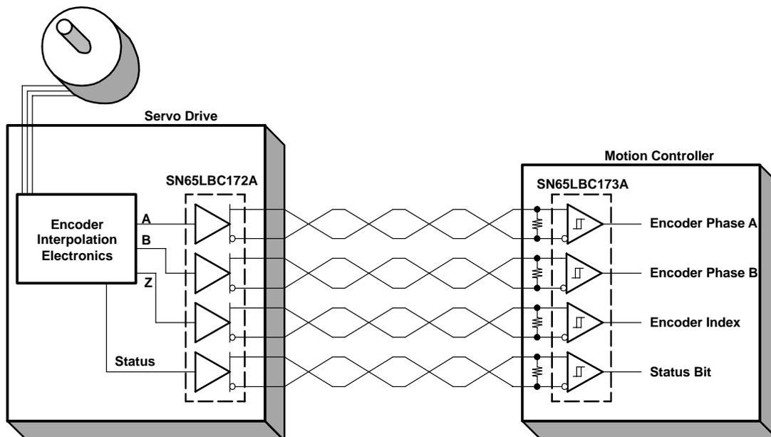
**Figure 7. Typical Application, Encoder Feedback Signals**
