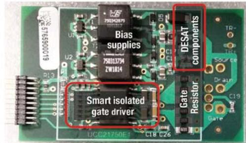
Integrated features of smart isolated gate drivers enable:
