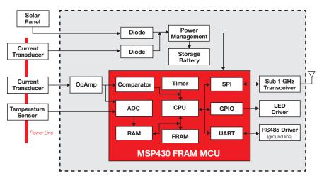
Figure 3. Functional block diagram of a smart fault indicator based on MSP430 FRAM MCU
