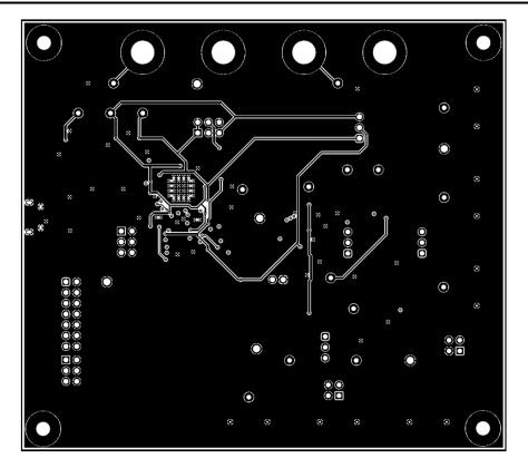
Figure 4-5. AFE881H1EVM PCB Mid Layer 2 Layout (GND Pour with Signal Routing)
