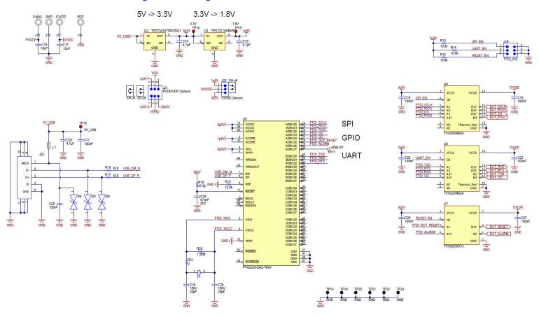
Figure 4-1. AFE881H1EVM Schematic: FTDI Controller
