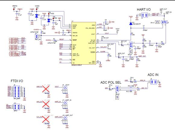
Figure 4-2. AFE881H1EVM Schematic: AFE881H1 I/O
