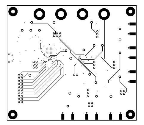
Figure 4-6. AFE881H1EVM PCB Bottom Layer Layout
