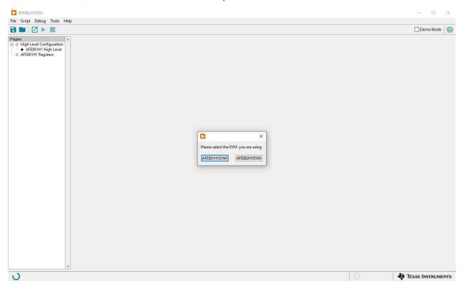
Figure 3-4. AFE88xH1EVM GUI Device Selection
