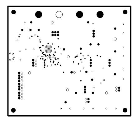
Figure 4-4. AFE881H1EVM PCB Mid Layer 1 Layout (GND Plane)
