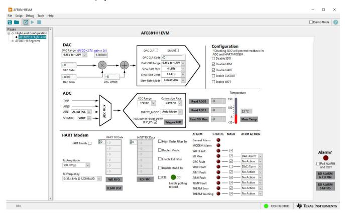
Figure 3-7. AFE881H1 High Level Tab
