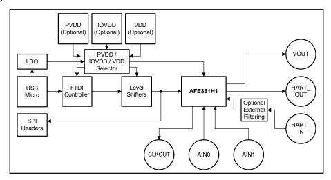
Figure 2-1. Block Diagram for the AFE881H1EVM
