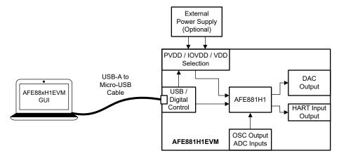
Figure 2-3. AFE881H1EVM Hardware Setup
