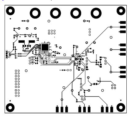
Figure 4-3. AFE881H1EVM PCB Top Layer Layout
