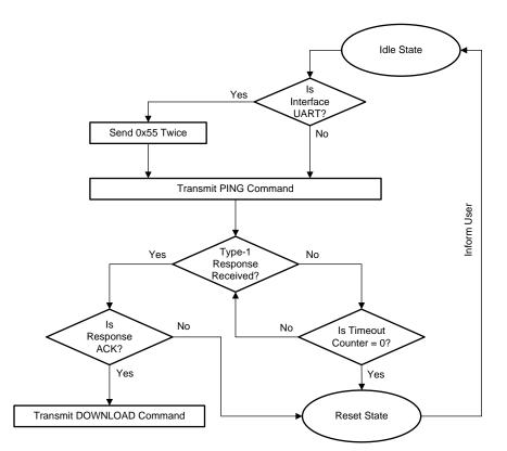
Figure 11. Serial Protocol Sequence-1
