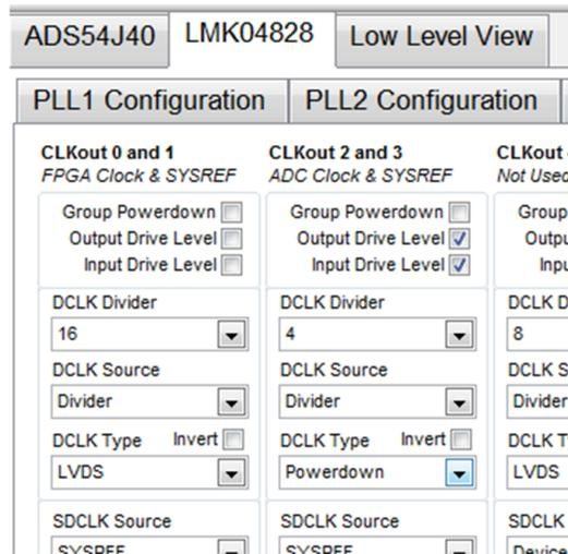
Figure 10. LMK04828 Clock Outputs Tab
