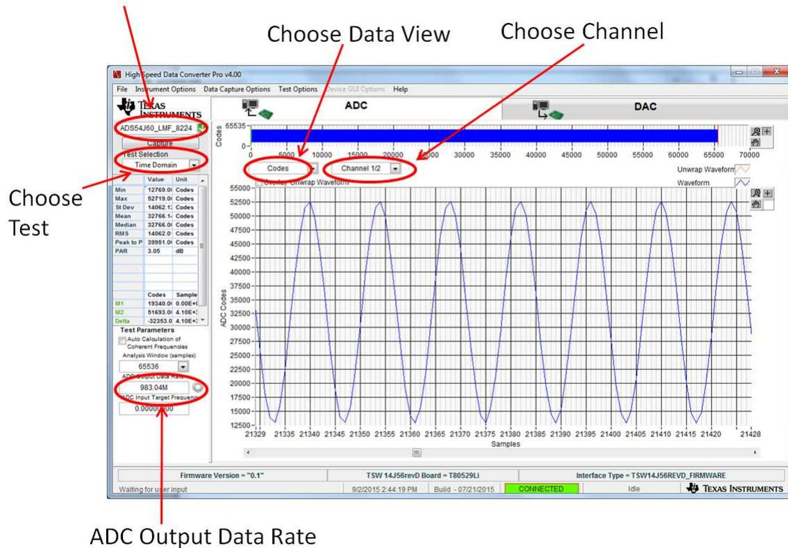
**Figure 5. HSDC Pro GUI Main Panel**
