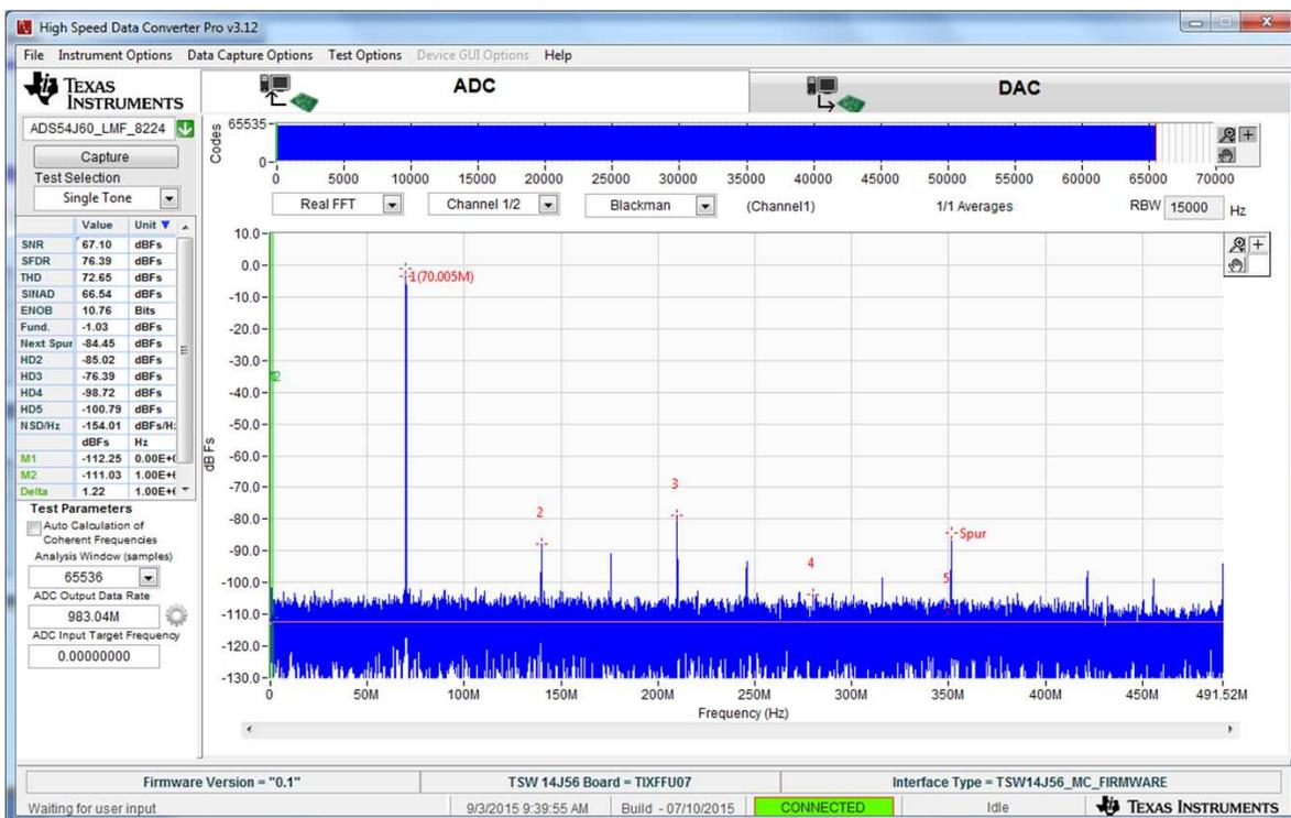
Figure 7. Channel 1 (LMH3401) Data Capture Results from Quick Start Procedure
