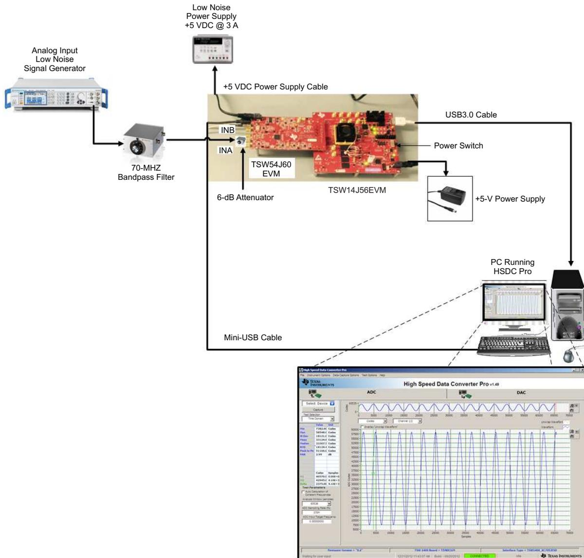
Figure 2. Quick Start Test Setup
