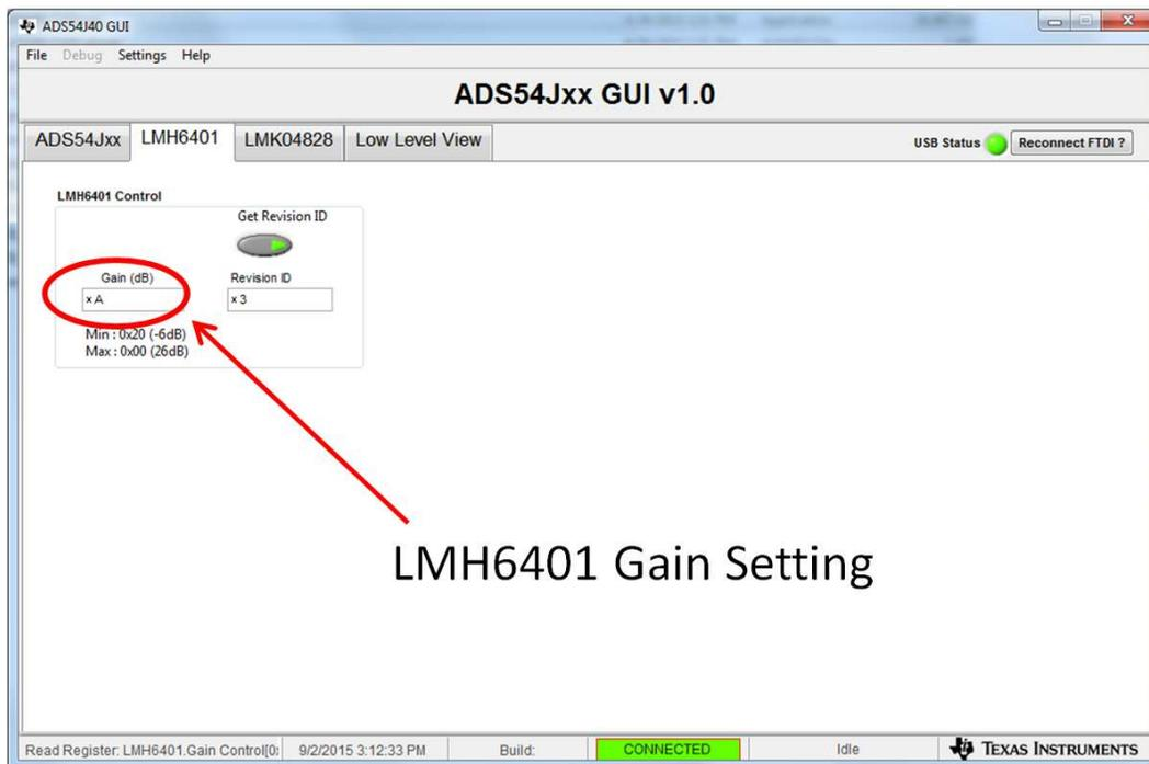
**Figure 4. LMH6401 Gain Setting Control**
